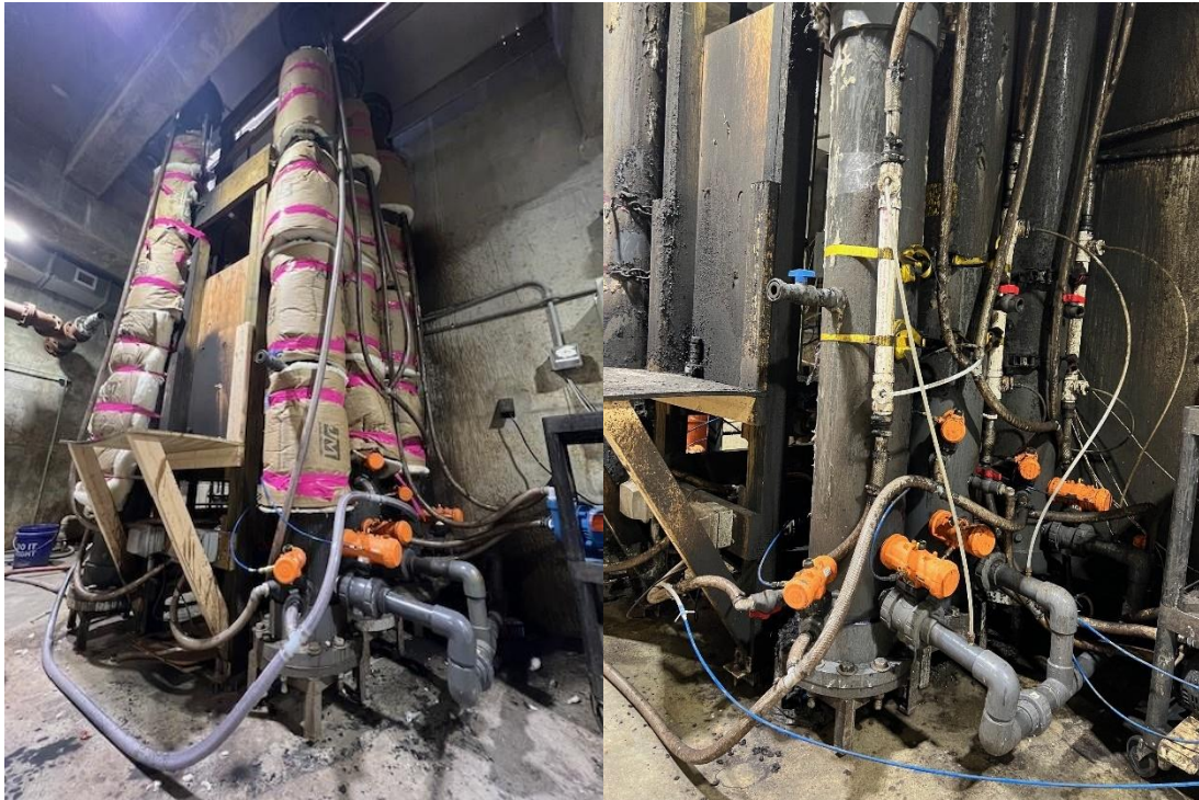
Figure 70: Pilot temperature control via insulation added for the winter months and NPW heat exchangers for the summer months.
