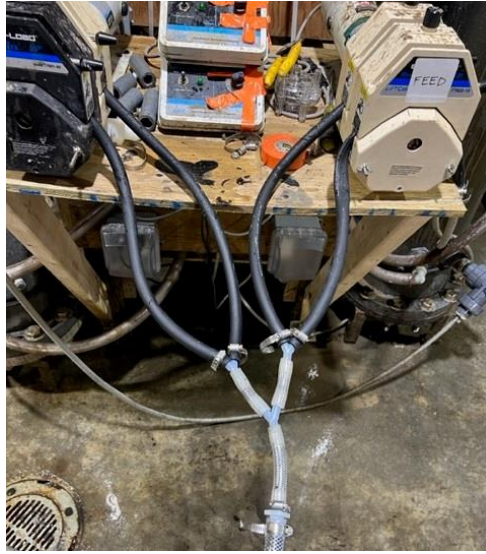
Figure 64: Pilot feed flow setups - the second continuous feed iteration with ½-inch tubing and Y-fittings.
