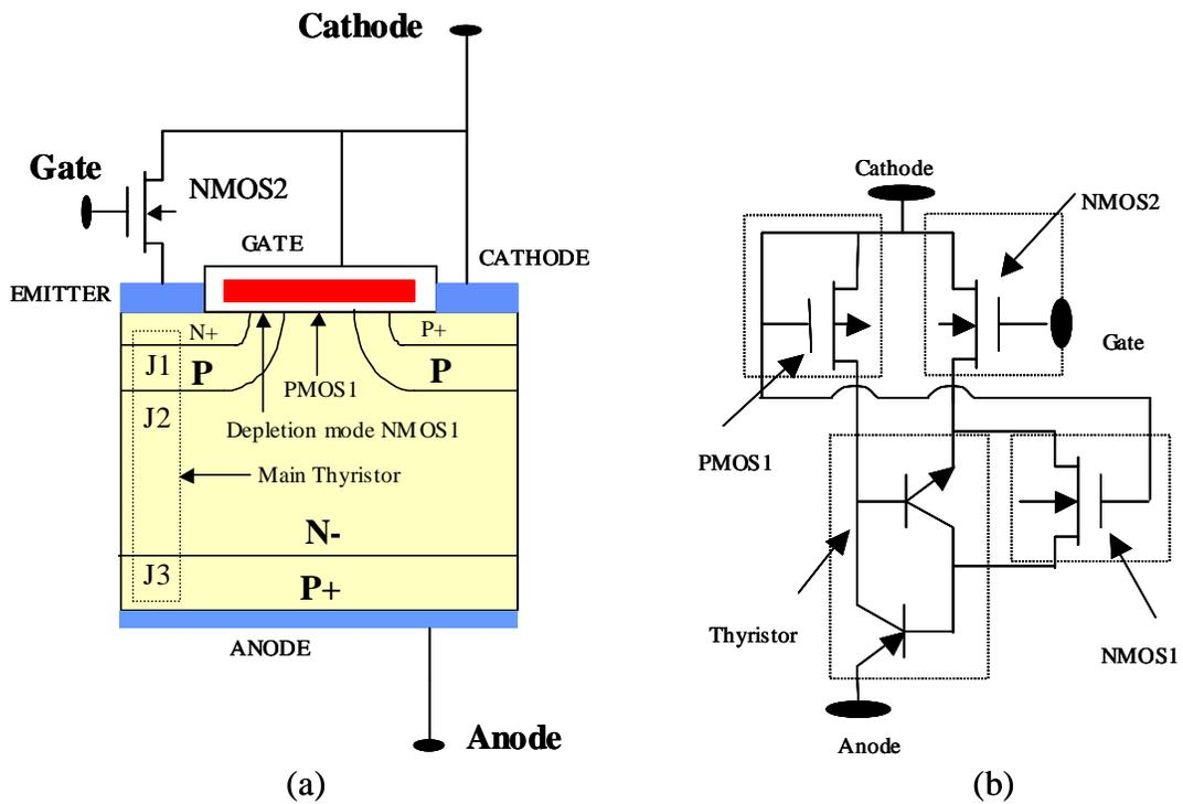
Fig. 2.20 The cross-section view of the ECT with external emitter switch FET (a) and its equivalent circuit (b).
