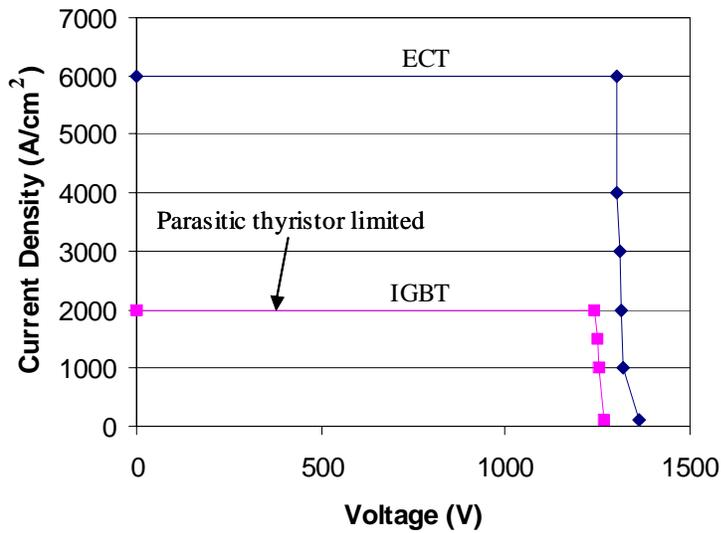
Fig. 3.10 Simulated RBSOA of the ECT in comparison with the RBSOA of the IGBT.
