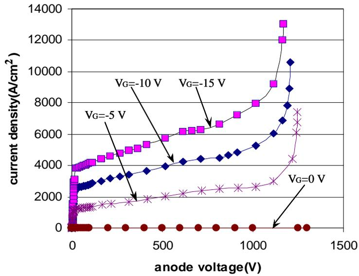
Fig. 3.5 The output characteristics of the ECT obtained by device simulation.
