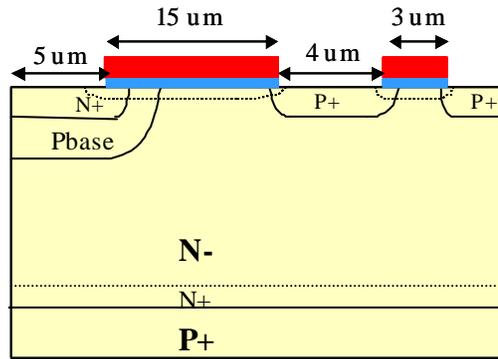
Fig. 3.16 The dimensions of the ECT unit cell.
