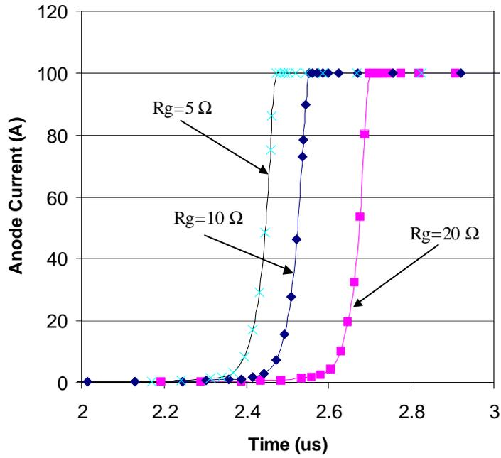
Fig. 3.13 The ECT turn-on waveforms with different gate resistance.
