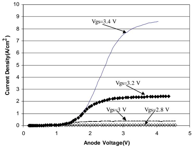
Fig. 4.17 The output characteristics of the fabricated device.
