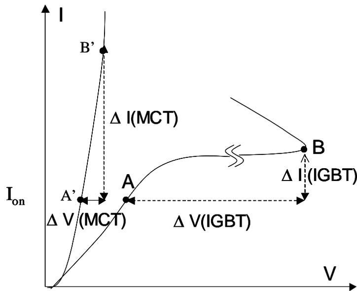
Fig. 2.16 The difference between what occurs in the gate delay cells of the MCT and that of the IGBT when the anode voltage rises.
