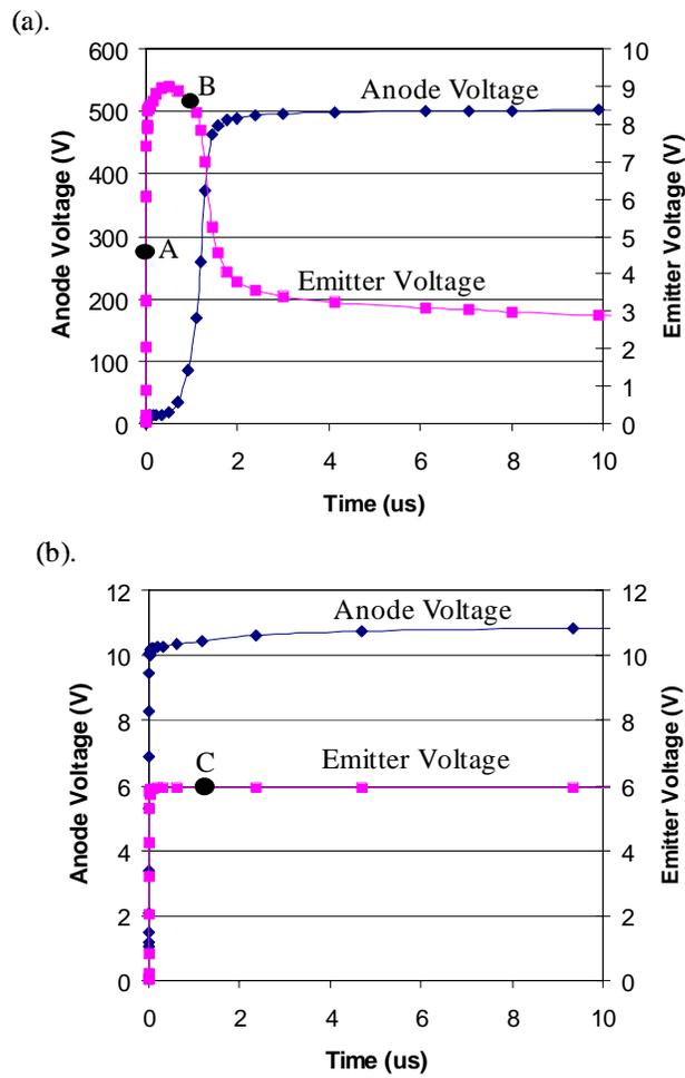
Fig. 4.24 The current and voltage waveform during turn-off (a) successful turn-off (b) turn-off failed.
