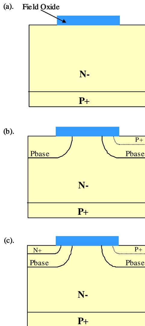
Fig. 4.14 Major steps of the HECT fabrication process.
