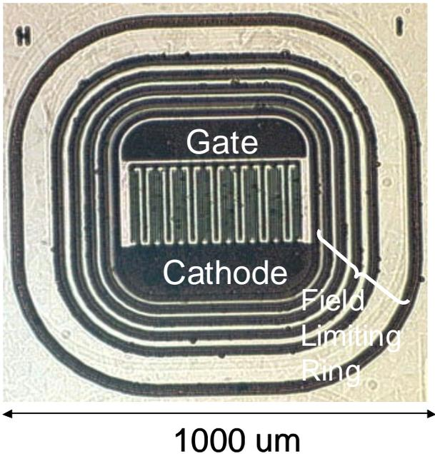
Fig. 3.15 The test structure of ECT with gate length of 3  $\mu\text{m}$  and width of 1500  $\mu\text{m}$ .
