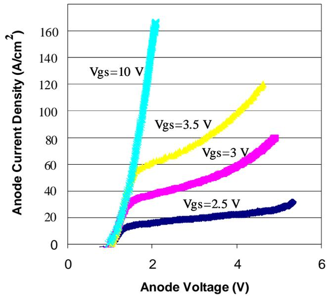
Fig. 3.21 Experimental output characteristics of the IGBT.
