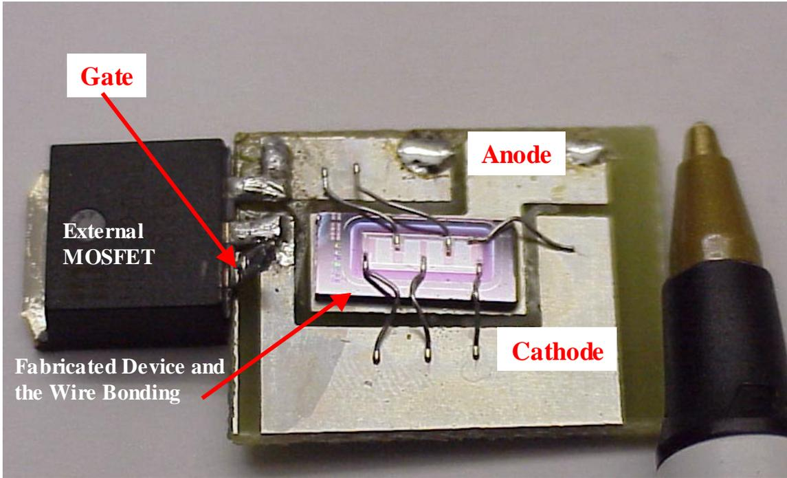
Fig. 4.15 The overall structure of the HECT after packaging.
