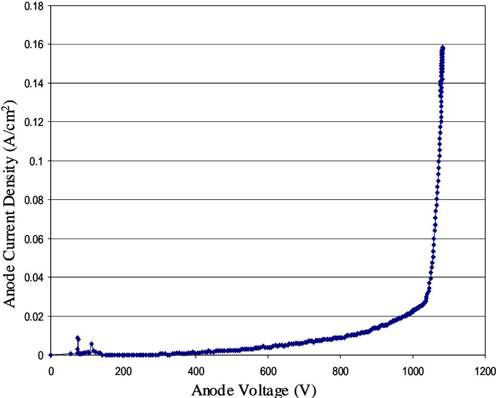
Fig. 3.19 The measured breakdown voltage of the ECT.
