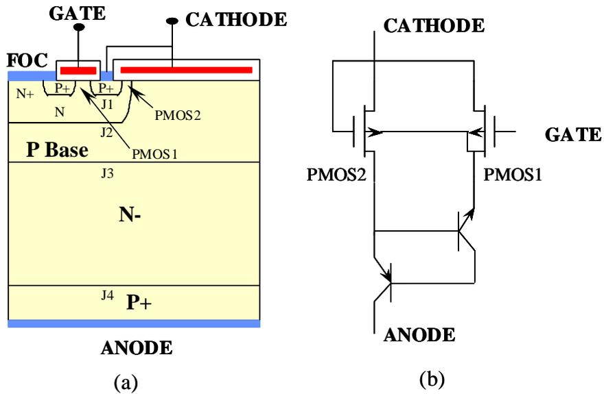
Fig. 2.17 The cross-section view of the ECT (a) and its equivalent circuit (b).
