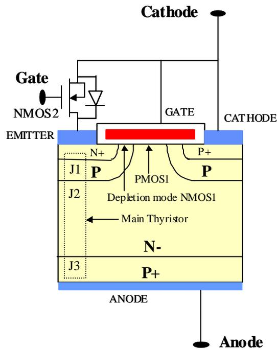
Fig. 4.2 The overall structure of the HECT.
