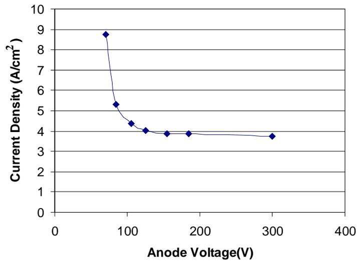
Fig. 4.23 The measured RBSOA of the HECT.
