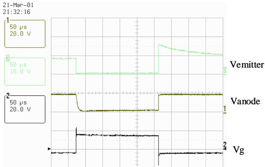
Fig. 4.21 The voltage waveform during switching.
