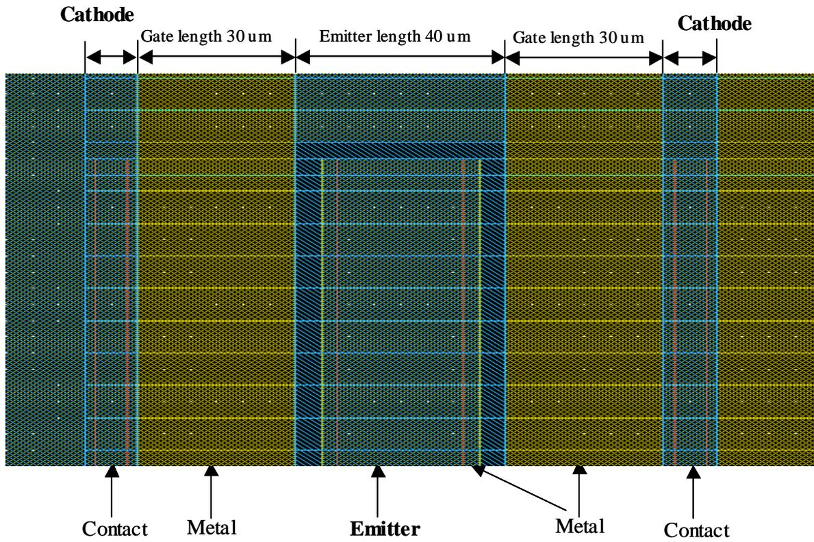
Fig. 4.9 Basic cell dimension of the test structure.
