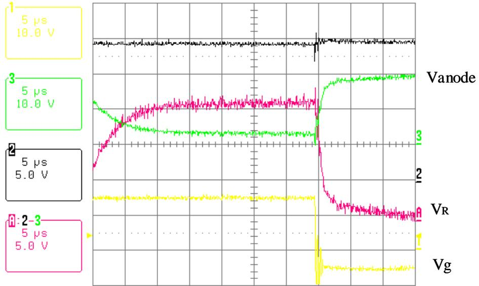
Fig. 4.22 The voltage waveform during turn-off.
