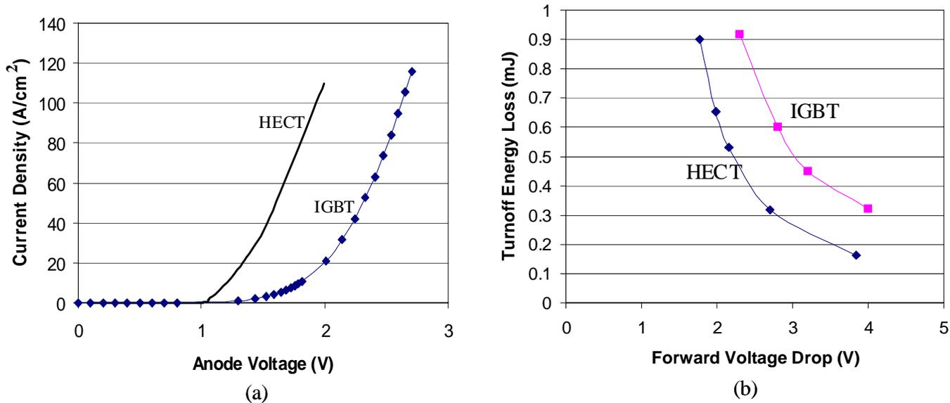
Fig. 4.3 Forward I~V characteristics (a) and technology trade-off curve (b) of the 4K V HECT comparing with that of the IGBT.
