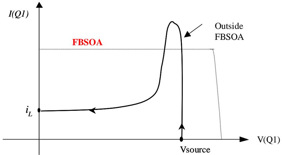
Fig. 2.5 The voltage-current trajectory of Q1 during its turn-on (large current overshoot exists due to diode D2 reverse recovery).
