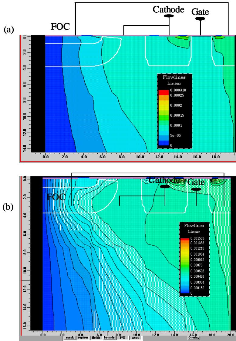
Fig. 3.6 The current flowlines of the ECT (a) in the forward conduction mode and (b) in the high voltage current saturation mode.
