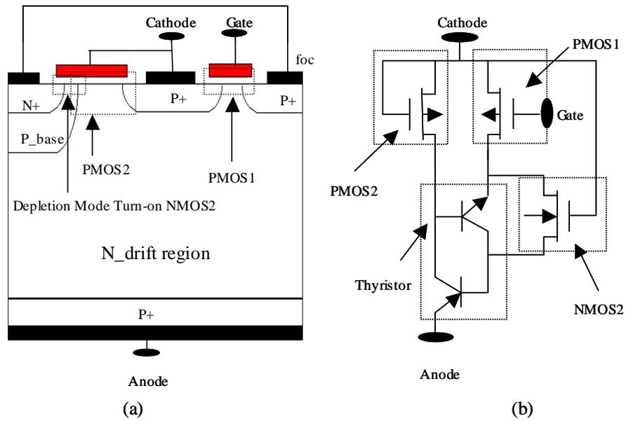
Fig. 2.19 The cross-section view of the ECT with a p-channel emitter switching FET (a) and its equivalent circuit.
