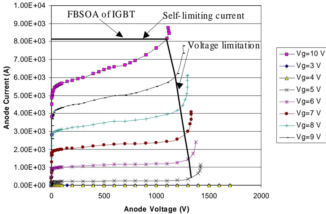
Fig. 2.7 An IGBT forward I~V characteristics showing the definition of the FBSOA determined by the avalanche voltage at high current (this FBSOA is only achievable in small pulse condition).
