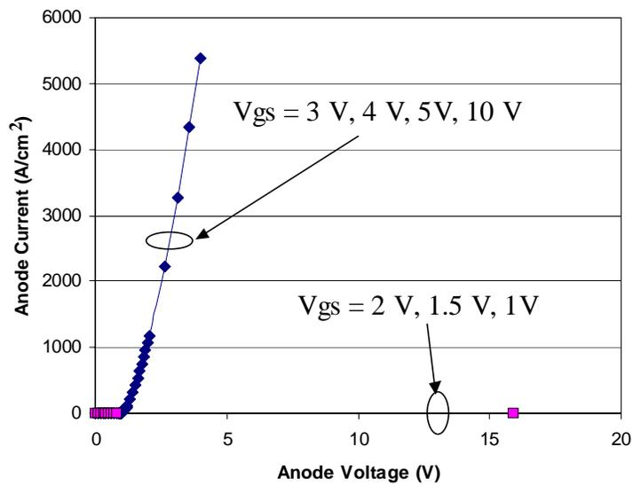
Fig. 2.13 The output characteristics of the MCT.
