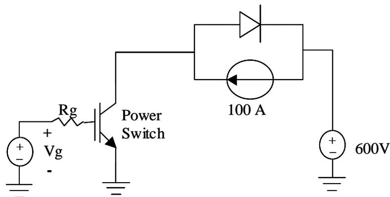
Fig. 3.12 Turn-on circuit with varying gate resistor used in the simulation.
