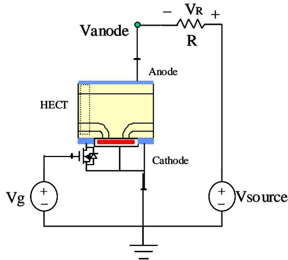
Fig. 4.20 Test circuit used to perform the resistive load switching test.
