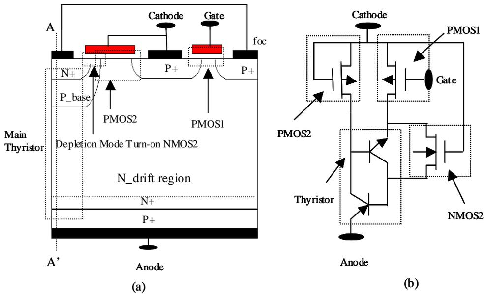
Fig. 3.1 Device structure of the three terminal ECT (a) and its equivalent circuit (b).
