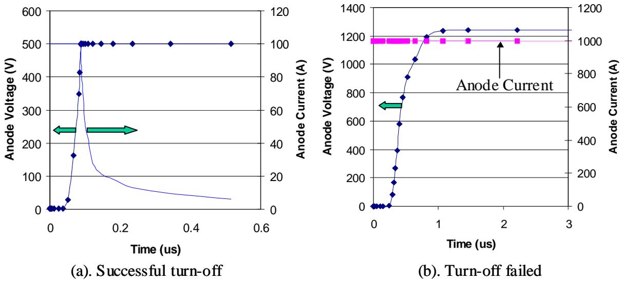
Fig. 3.9 The voltage and current waveform during turn-off.
