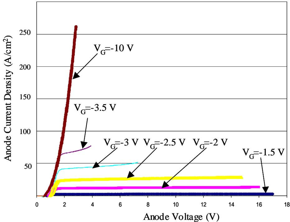
Fig. 3.20 Experimental output characteristics of the ECT.
