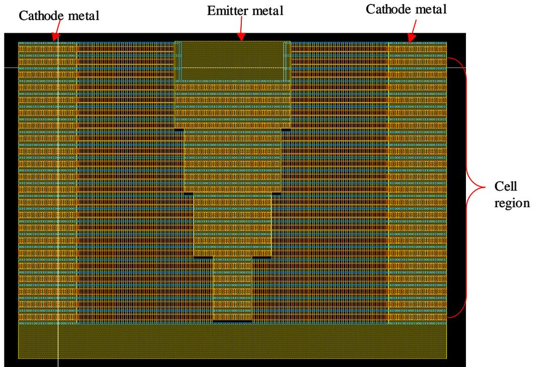
Fig. 4.8 The row cell of the test structure.
