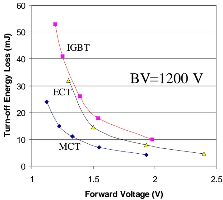
Fig. 3.11 Tradeoff between forward voltage drop and the turn-off loss per cycle when the current density is 100 A/cm<sup>2</sup> and turn-off voltage is 600 V.
