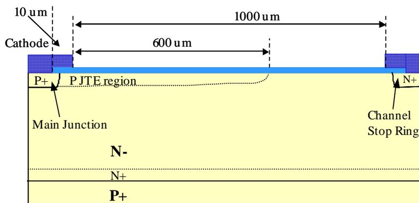
Fig. 4.10 The cross-section view of the JTE termination region.
