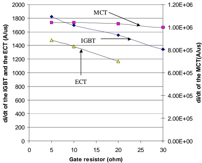
Fig. 3.14 The  $di/dt$  of the ECT at different gate resistor comparison with that of the IGBT and the MCT.
