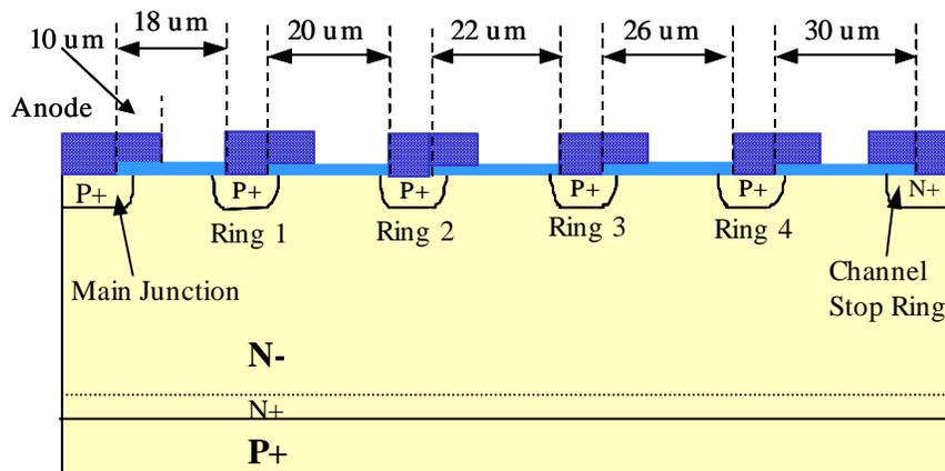
Fig. 3.17 The cross-section view of the ECT edge termination region.
