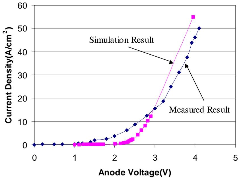
Fig. 4.16 The forward I~V curve of the fabricated device.
