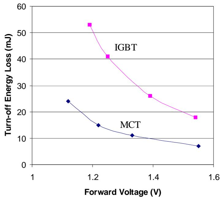
Fig. 2.15 Tradeoff between forward voltage drop and the turn-off loss per cycle when the current density is 100 A/cm<sup>2</sup> and turn-off voltage is 600 V.
