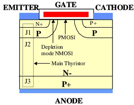
Fig. 4.1 The cross-section view of the high voltage part of the HECT and IGBT.
