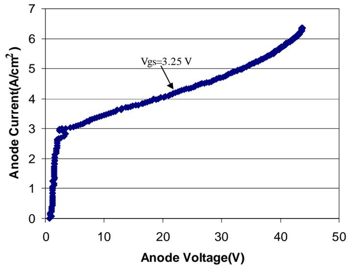
Fig. 4.18 The output characteristics of the fabricated device at high anode voltage.
