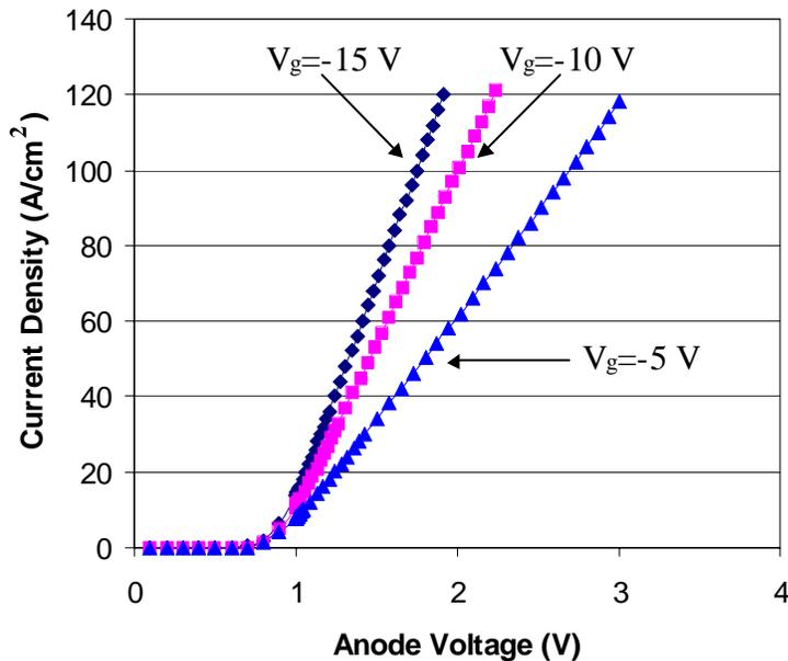
Fig. 3.3 The forward I~V characteristics of the 1200 V ECT obtained by device simulation.
