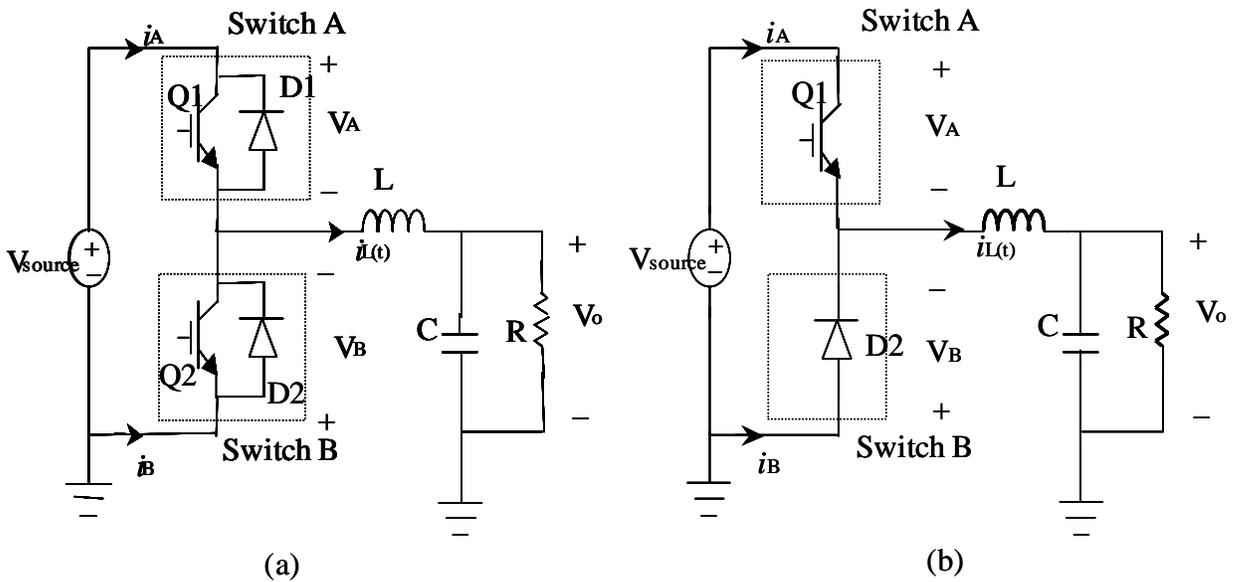
Fig. 2.2 The circuit realization branch in the dc-3φac inverter system (a) the transistor realization and (b) the simplified circuit when the load current is positive .
