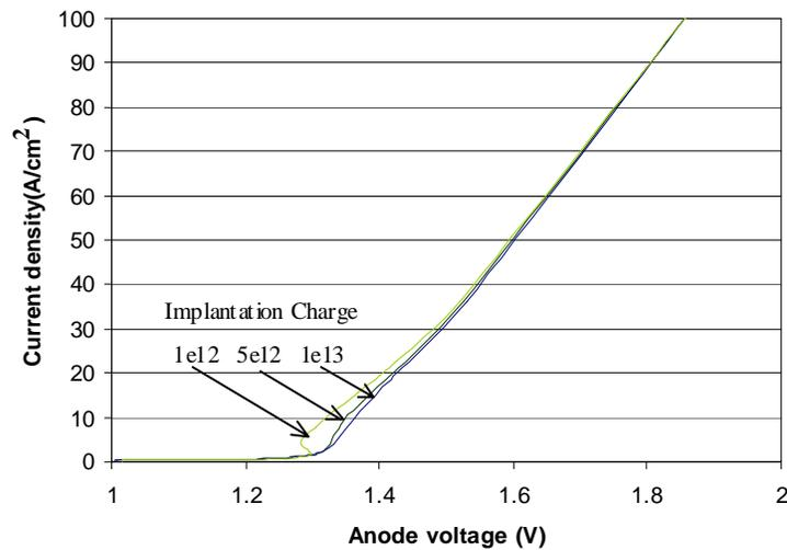
Fig. 4.13 The anode voltage and current curves at different threshold voltage adjustment implantation charges.
