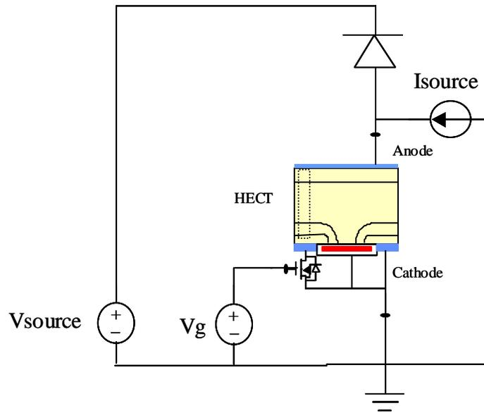
Fig. 4.5 Schematic of the simulation circuit to calculate the RBSOA.
