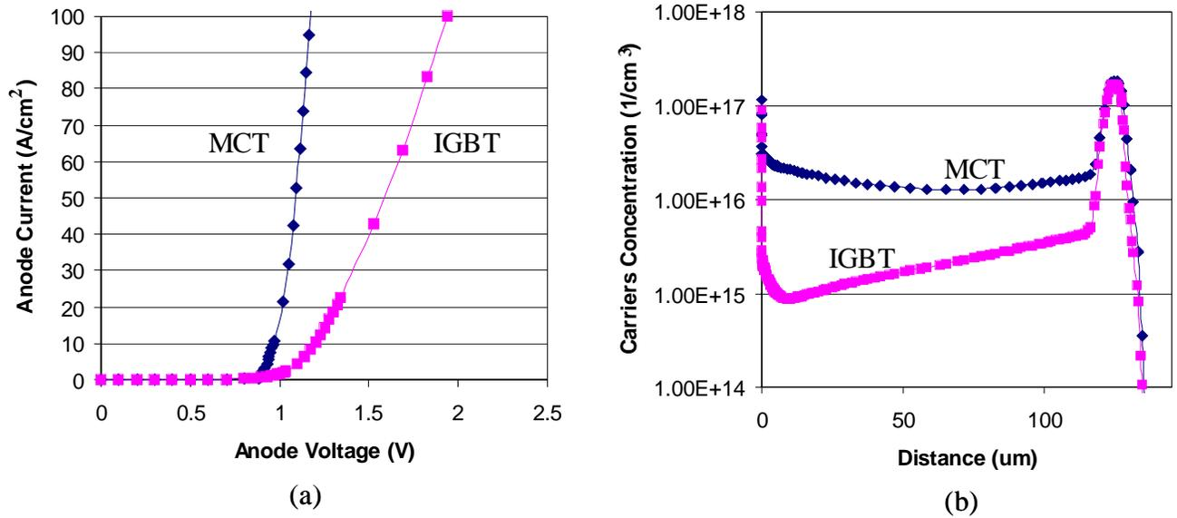
Fig. 2.14 The forward voltage drop (a) and the typical carriers concentration distribution (b) of 1200 V MCT when the current density is 100 A/cm<sup>2</sup> comparing with the IGBT.
