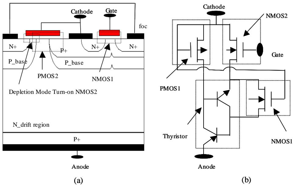
Fig. 2.18 The cross-section view of the ECT with an n-channel emitter switching FET (a) and its equivalent circuit.
