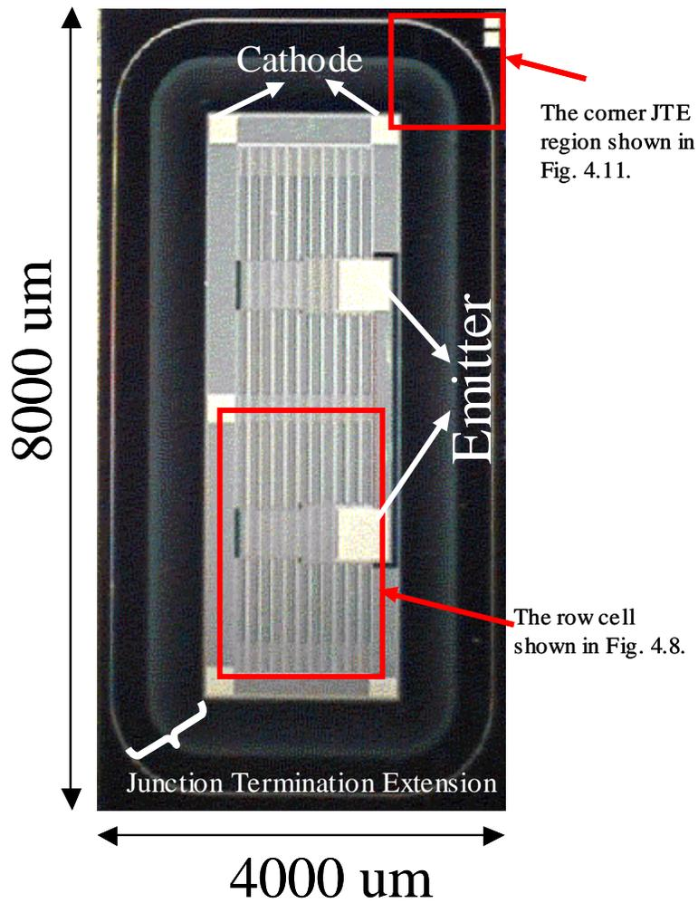
Fig. 4.7 The test structure of HECT with gate length of 30  $\mu\text{m}$ .
