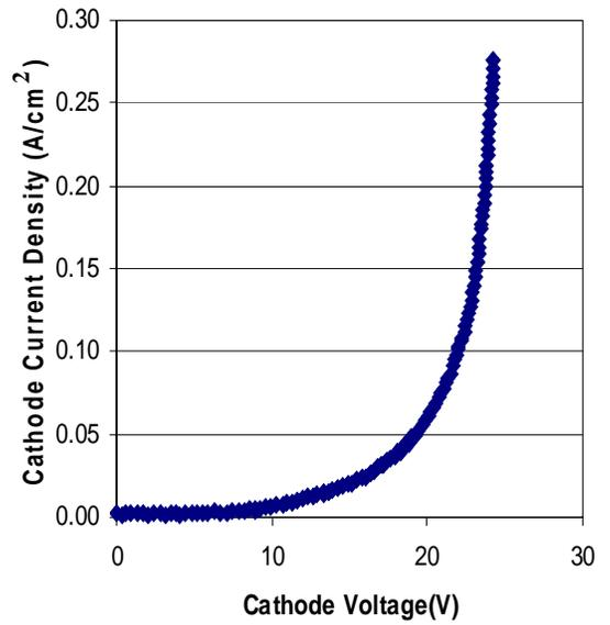
Fig. 4.19 The breakdown voltage between the anode and the cathode (a) and the breakdown voltage between the cathode and the emitter (b).
