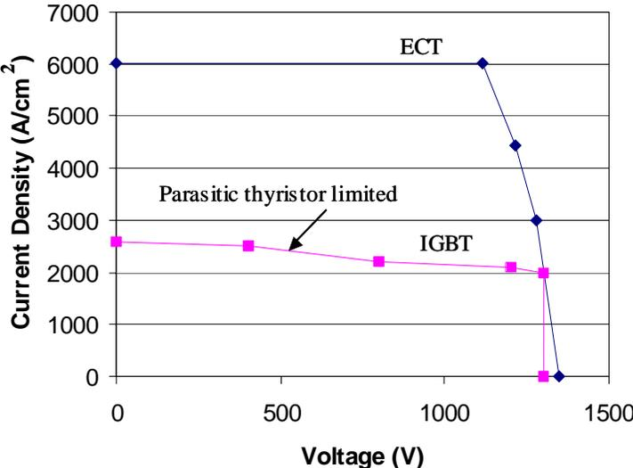
Fig. 3.7 The FBSOA of the ECT in comparison with the FBSOA of the IGBT.
