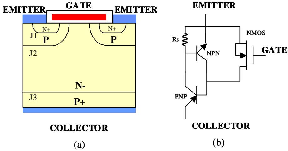
Fig. 2.9 The cross-section view of the IGBT (a) and its equivalent circuit (b).
