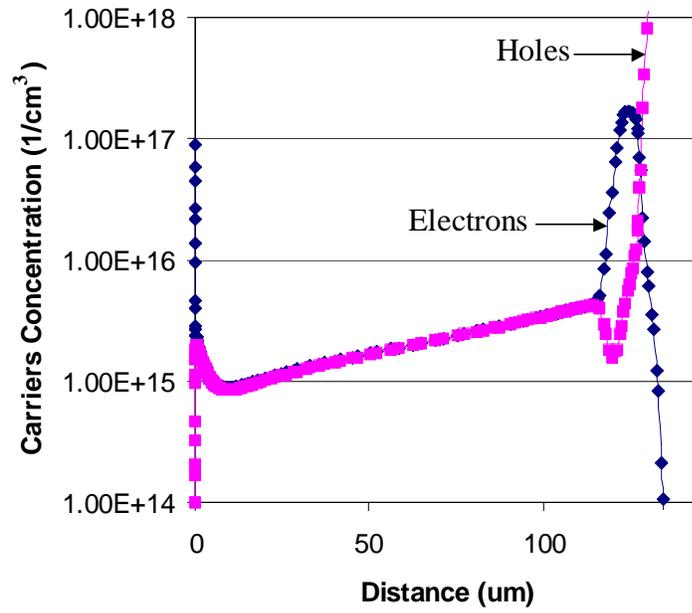
Fig. 2.11 Typical carriers distribution of a 1200 V IGBT when the current density is  $100 \text{ A/cm}^2$  shown in Fig. 2.10 as point A.
