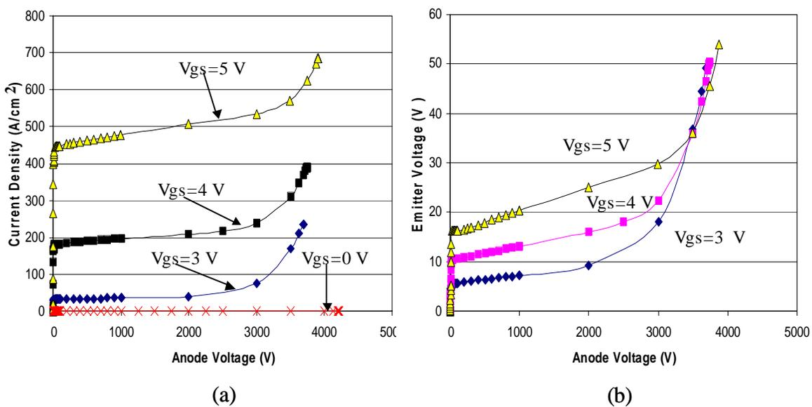
Fig. 4.4 The output characteristics of the HECT (a) and the emitter voltage (b).
