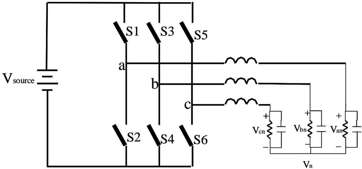
Fig. 2.1 The dc-3φac inverter system.
