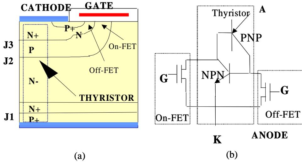
Fig. 2.12 The cross-section view of the MCT (a) and its equivalent circuit (b).
