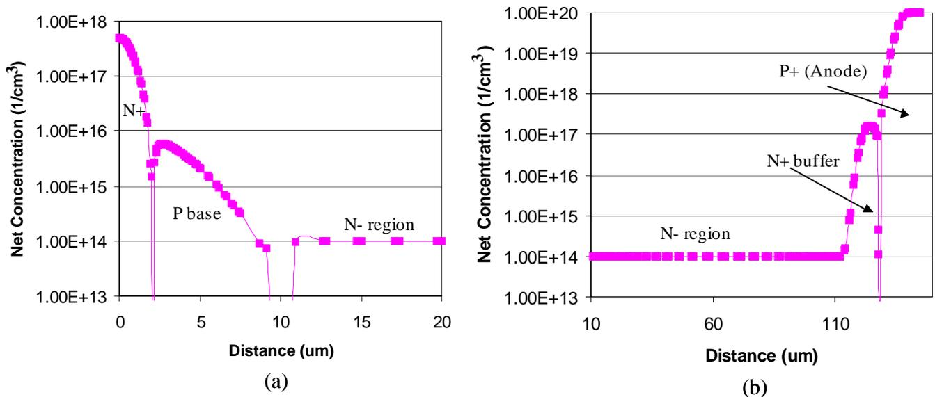
Fig. 3.2 1-D doping profile of the top cell (a) and anode region (b) of the 1200 V ECT along the cut line of AA' shown in Fig. 3.1.
