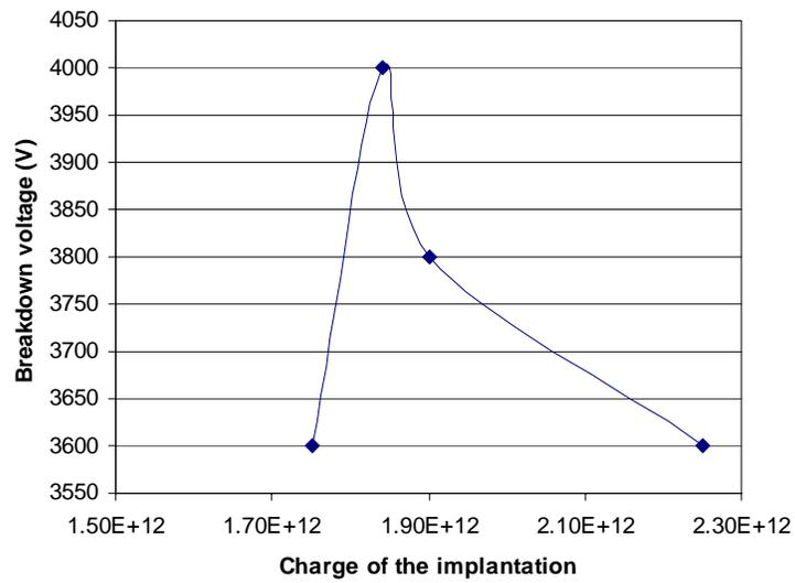
Fig. 4.12 The breakdown voltage at different implantation charge of the JTE.
