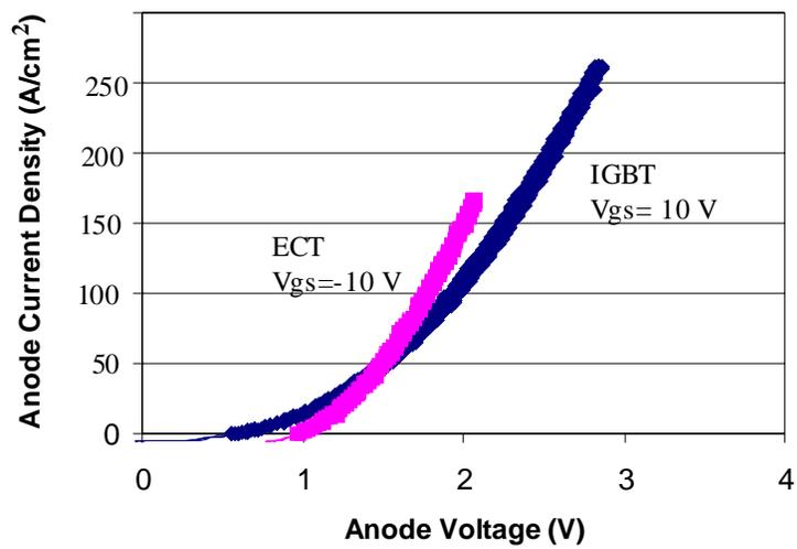
Fig. 3.22 Experimental forward voltage drop of the ECT comparing with the IGBT.
