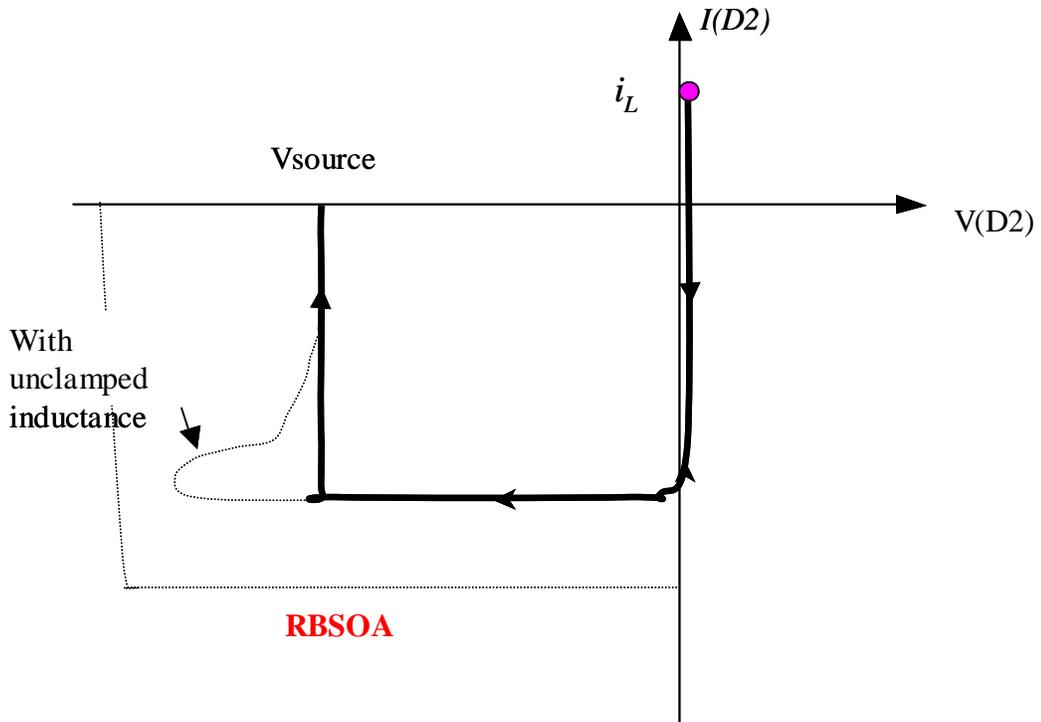
Fig. 2.6 The diode D2 trajectory during its turn-off (a definition of RBSOA can be made for the diode and the effect of unclamped inductance will result in voltage overshoot).
