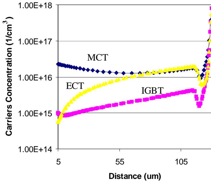
Fig. 3.4 The typical carriers concentration distribution of 1200 V ECT when the current density is 100 A/cm<sup>2</sup> comparing with that of the IGBT and MCT.
