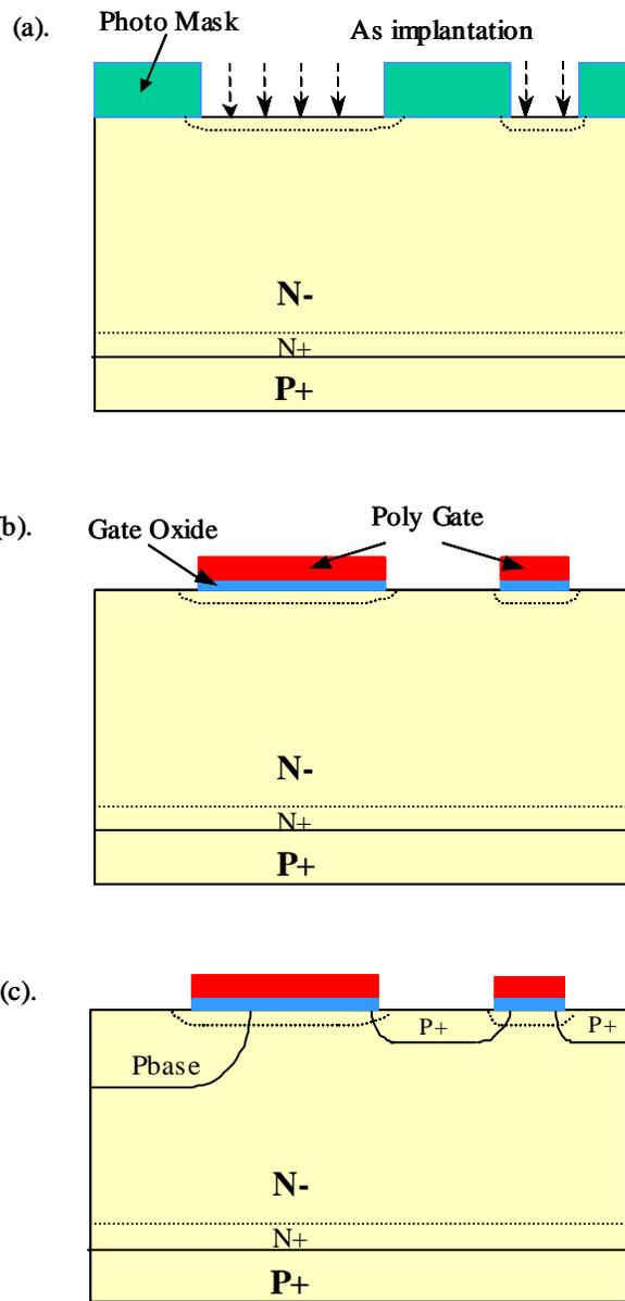
Fig. 3.18 Major steps of the proposed ECT fabrication process.
