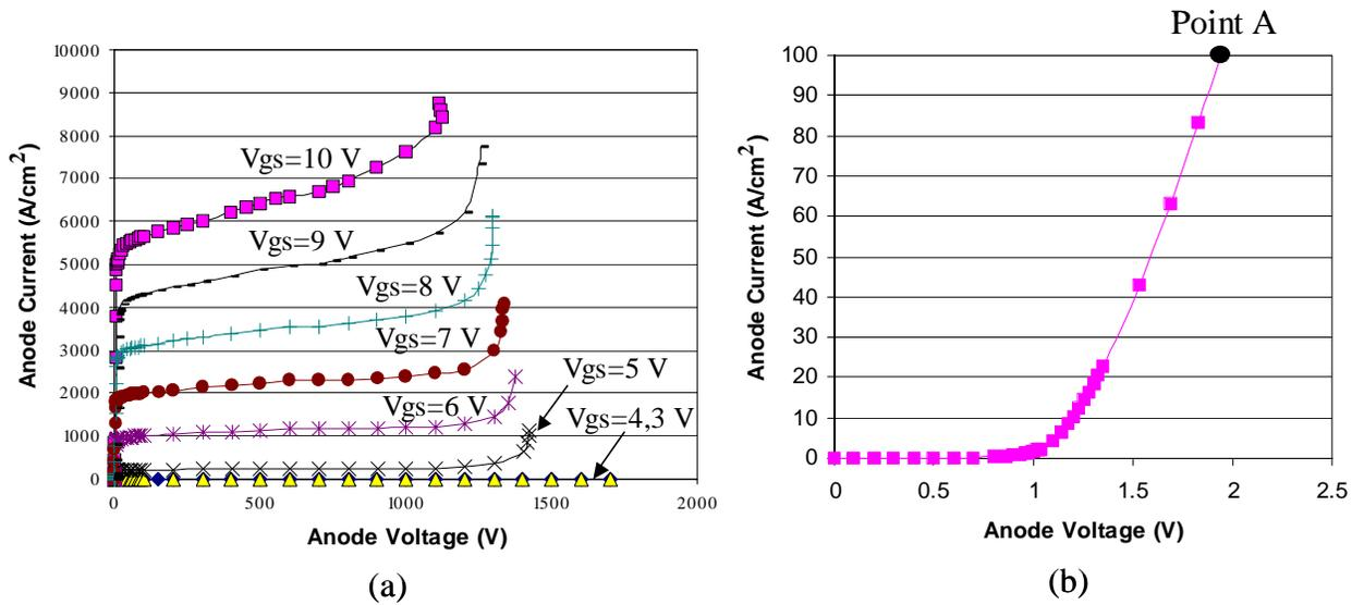
Fig. 2.10 The IGBT output characteristics of the high voltage current saturation region (a) and the low voltage region (b).
