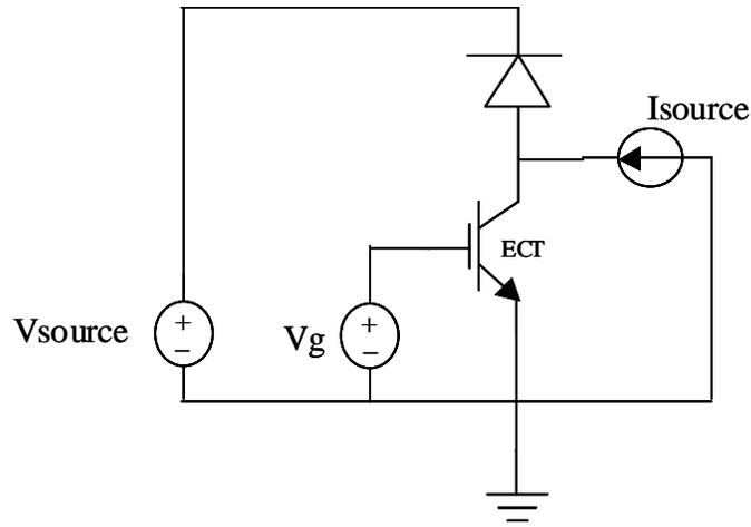
Fig. 3.8 Circuit diagram used to calculate the RBSOA using mixed mode MEDICI simulator.
