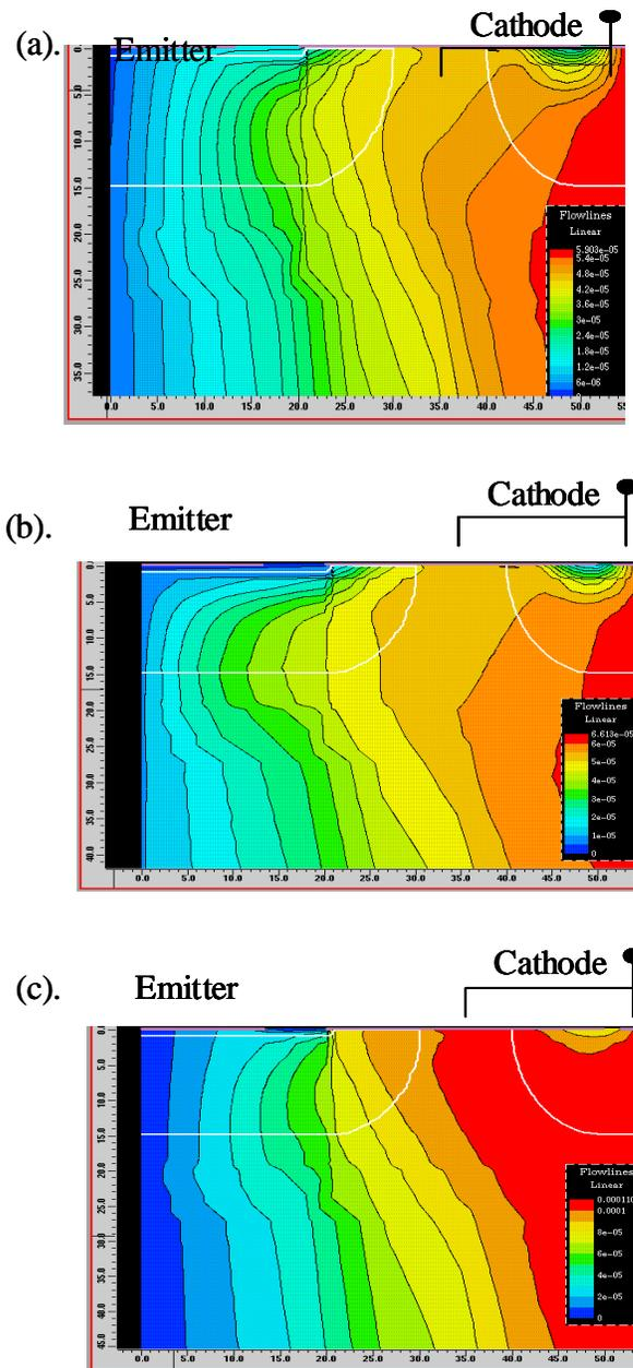
Fig. 4.25 The current flowlines of the HECT during turn-off corresponding to the point A,B,C shown in Fig. 4.24.
