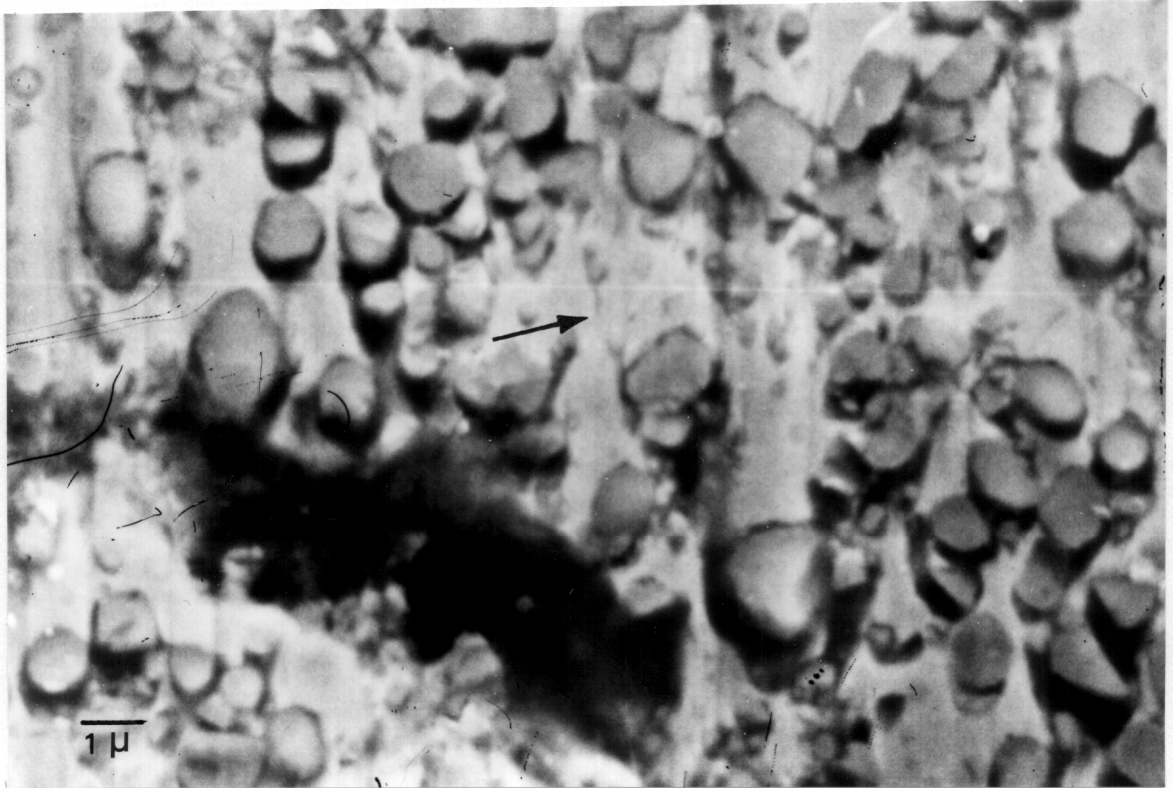
Figure 64: Cracks (arrow) in wear scar of ion nitrided CPM10V RC 55.
