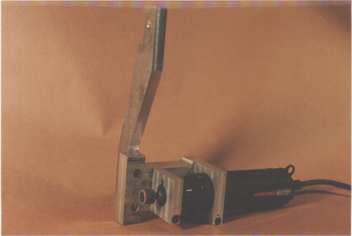
Figure 14: Grinding attachment for truing test wheels
