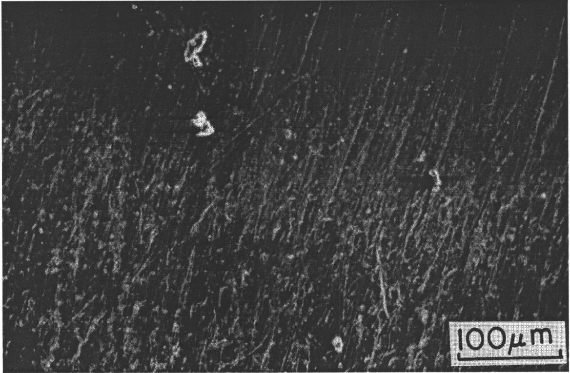
Figure 75: Transition in appearance of wear scar on ion nitrided Thyssen 4122.
