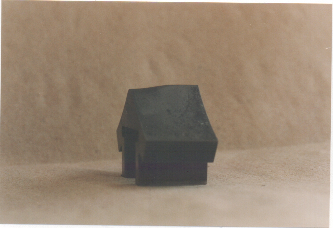
Figure 2: Worn saddle returned from service
