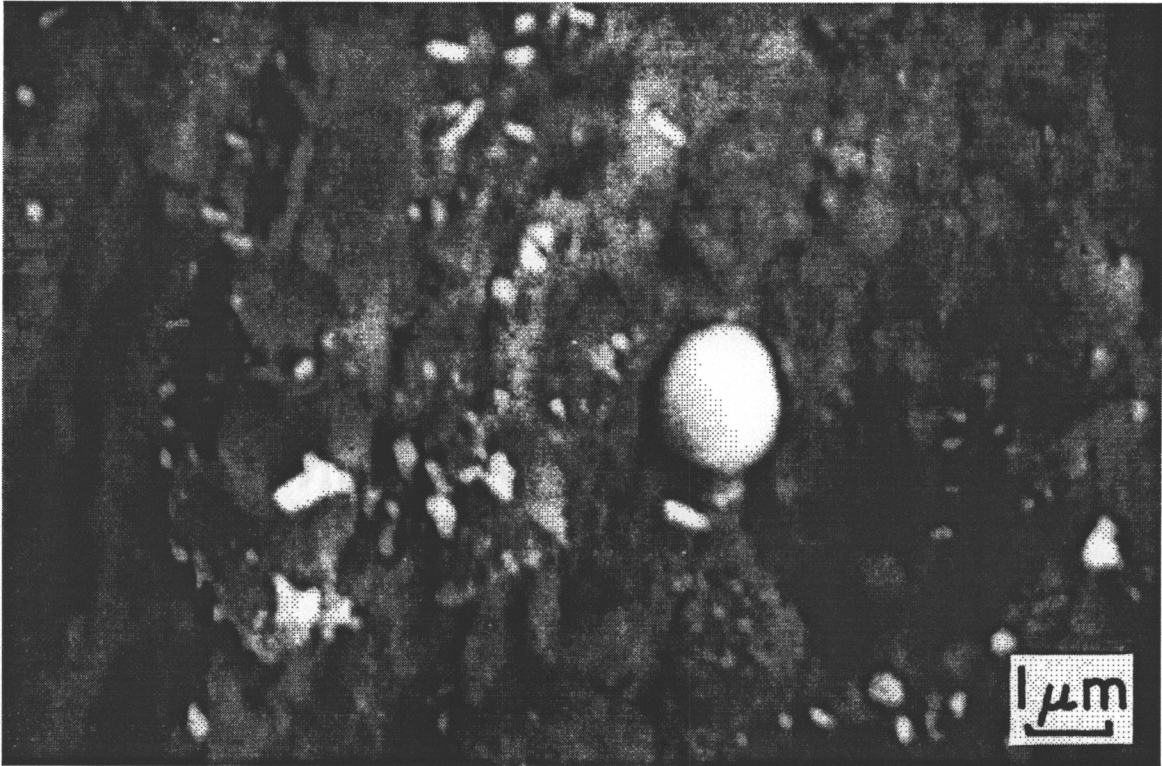
Figure 45: Wear sheet detaching from FerroTiC CM45 wear scar.
