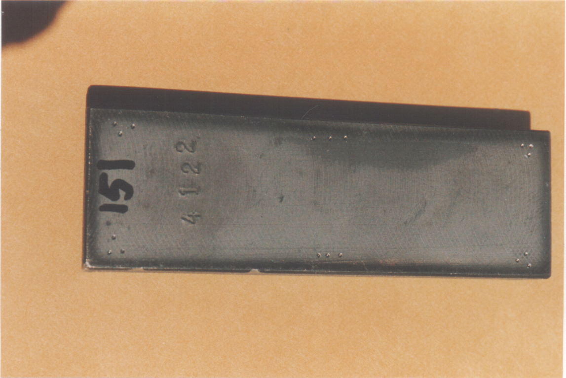
Figure 31: Typical surface appearance of Thyssen 4122 ion nitrided samples.
