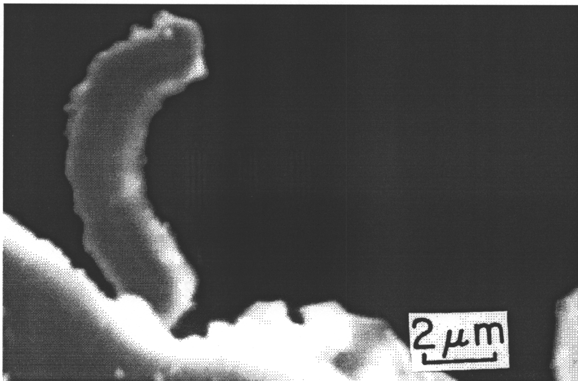
Figure 47: Microchip type particles in wear debris from FerroTiC CM45.
