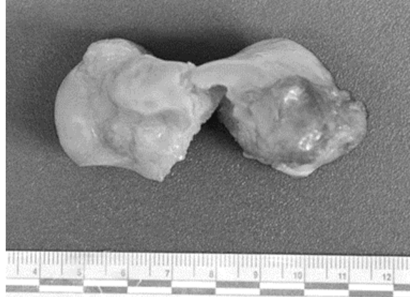
Figure 18: Fracture of the right talus of SB1C2 (5 th -percentile female). Medial view; right side of photo is posterior.
