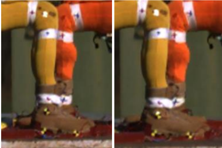
Figure 24: SB1 Crew 2 (yellow) right calcaneus fracture. Left photo: time-zero. Right photo: 3.5 ms from time-zero.
