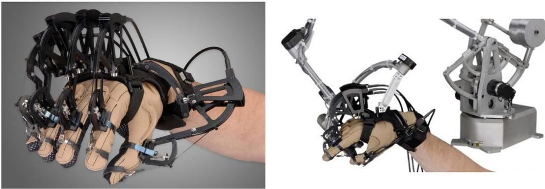
**Figure 2.6:** Picture of the CyberGrasp hand exoskeleton [36]
