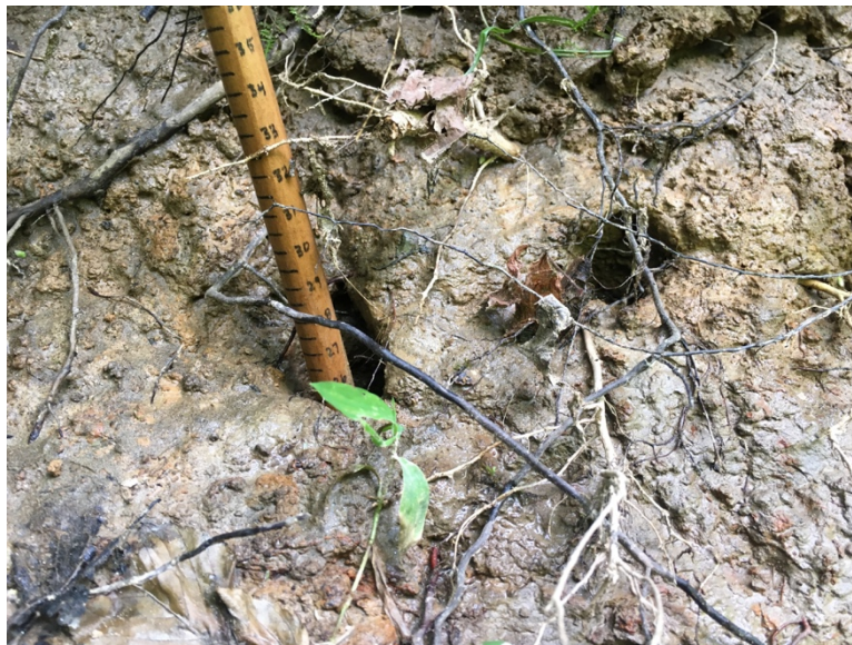
Figure A-5: Depth measurement of macropore using a modified wooden dowel with 0.5 cm increments. The same dowel was used to measure macropore elevation, width, and height.
