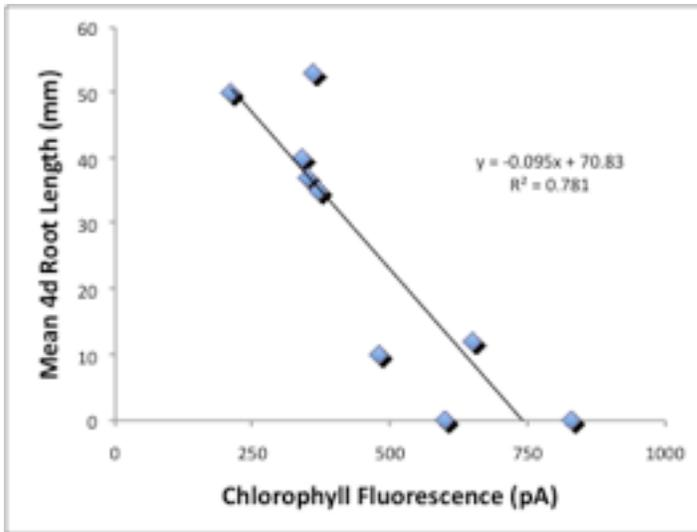
**Figure 4:** A linear regression of CF measured with a SeedMaster Analyzer from Fig. 3 versus mean 4 d root length in Fig. 2.
