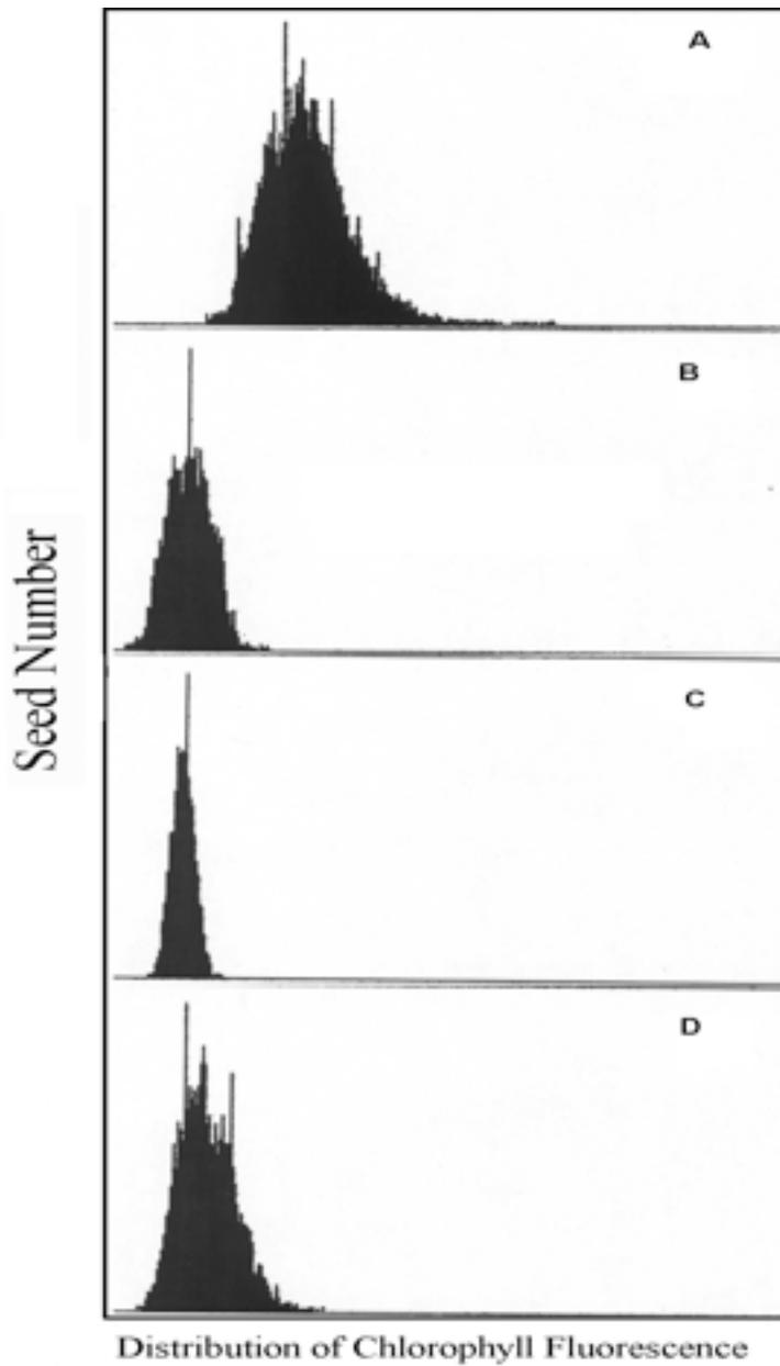
**Figure 5:** CF of ‘TopMark’ seeds harvested at different developmental stage, measured by a SeedMaster Analyzer. The relative scale of 0-1000 pA is the same for all three panels, and larger values represent greater fluorescence. (A) 35 DAA, (B) 45 DAA, (C) 55 DAA and (D) 65 DAA. Approximately 1000 ‘Top Mark’ seeds were measured at each stage of development. Amplitude is the number of seeds per CF frequency.
