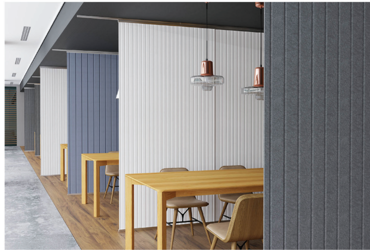
Acoustic sliding partitions can be used to separate the business incubator enclaves from the rest of the space and provide noise control.
