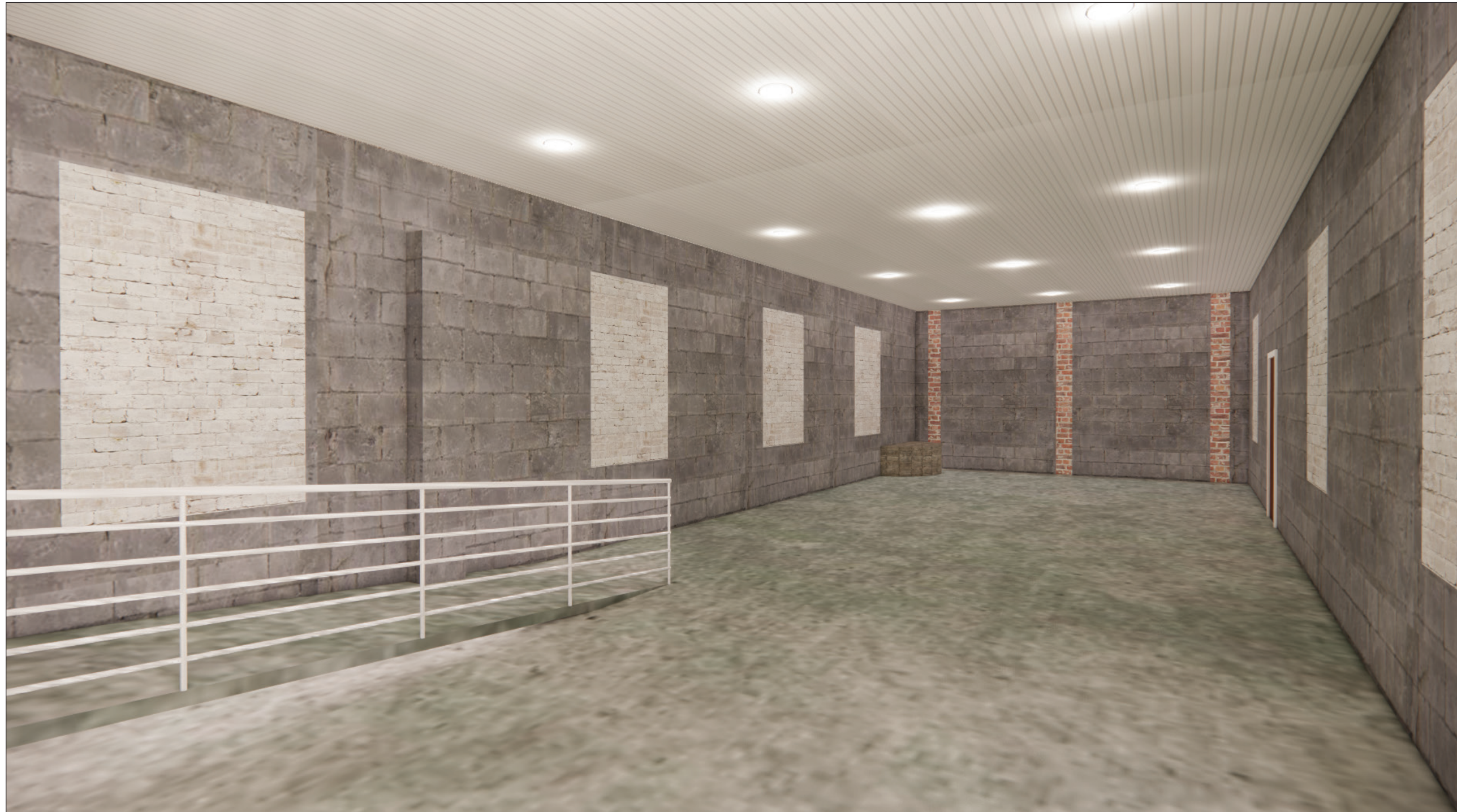
Perspective 3 (Vocational Shell): A ramp has been added to allow ADA access into the vocational area. The concrete block and brickwork from former Campbell County Training School students remain and windows remain blocked off.
