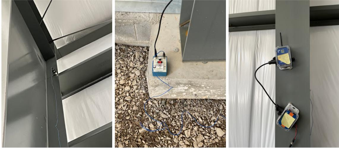
(a) Mounted accelerometer      (b) Signal conditioner      (c) XNode transmitter
