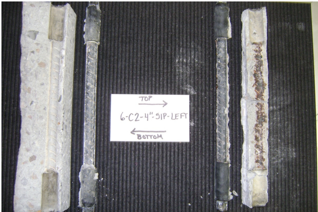
Figure E-2 – Specimen 6 – C-2 – 4” – SIP – Left – Bottom Side of both Bars
