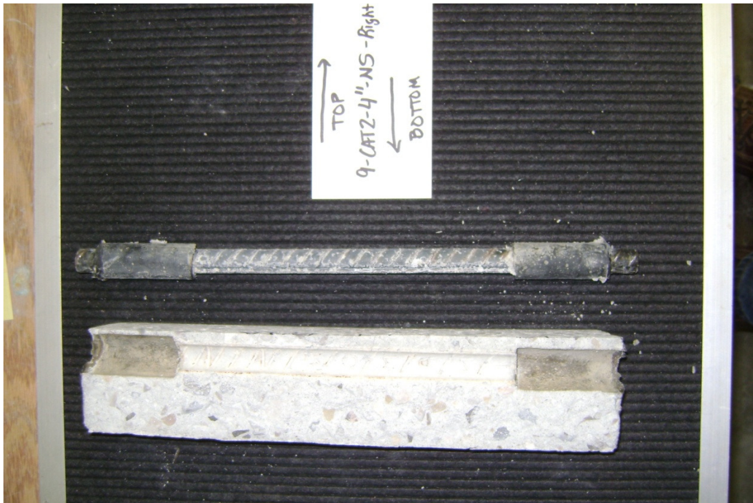
Figure E-12 – Specimen - 9 – C-2 – 4” – NSIP – Right – Top Side of Bottom Bar
