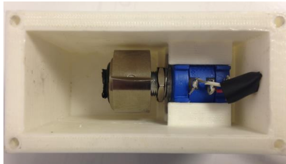
Figure 3.10 - Potentiometer securely placed inside the extensometer casing
