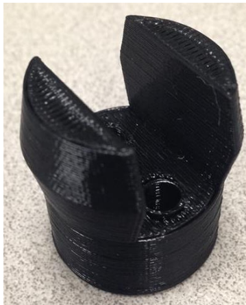
Figure 3.5 - 3-D printed borehole anchor
