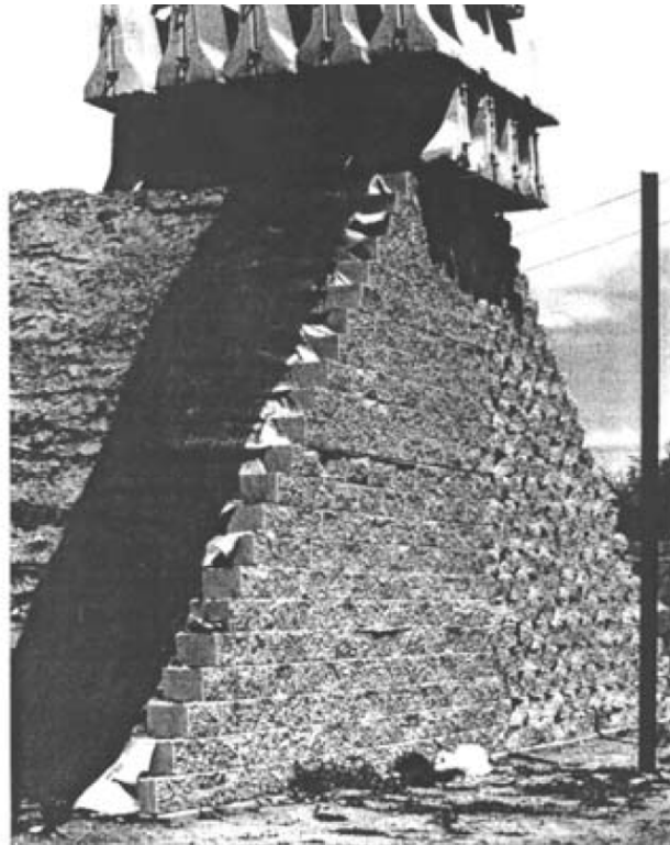
Figure 15: Commerce City Wall Experiment Wu, J. T. H. (2007). "Lateral Earth Pressure against the Facing of Segmental GRS Walls." Geosynthetics in Reinforcement and Hydraulic Applications (GSP 165) , Gabr, and Bowders (Eds.). ASCE, Reston, VA, 165-175. Used under fair use, 2014.
