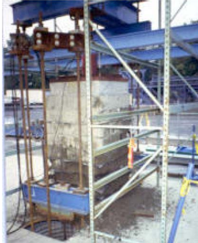
Figure 17: One of Five GRS Mini Pier Experiments Adams, M., Ketchart, K., and Wu, J. T. H. (2007a). "Mini Pier Experiments: Geosynthetic Reinforcement Spacing and Strength as Related to Performance." Geosynthetics in Reinforcement and Hydraulic Applications (GSP 165) , Gabr, and Bowders (Eds.), Reston, VA, 98-106. Use under fair use 2014.
