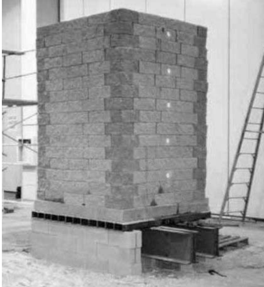
Figure 20: Vegas GRS Mini Pier after Testing Adams, M., Nicks, J., Stabile, T., Wu, J. T. H., Schlatter, W., and Hartmann, J. (2011a). "Geosynthetic Reinforced Soil Integrated Bridge System—Interim Implementation Guide." FHWA-HRT-11-026, Federal Highway Administration, McLean, VA. Used under fair use, 2014.
