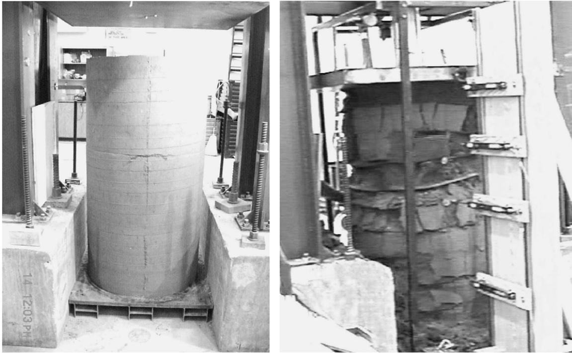
Figure 22: Test Setup Before and During Testing Elton, D. J., and Patawaran, M. A. B. (2004). "Mechanically Stabilized Earth Reinforcement Tensile Strength from Tests of Geotextile-Reinforced Soil." Transportation Research Board, Washington, D.C. Used under fair use, 2014.
