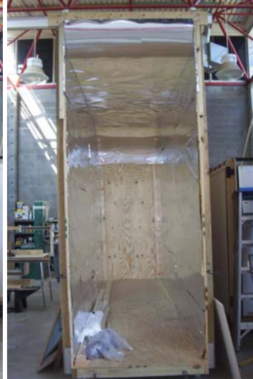
Figure 3.20: Attaching the corrugated cardboard layer, Durallar film, and the 3M prismatic sheets
