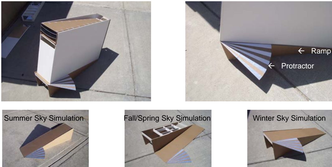
Figure 3.12: The ramp used to simulate seasonal solar altitudes with an equipped solar protractor
