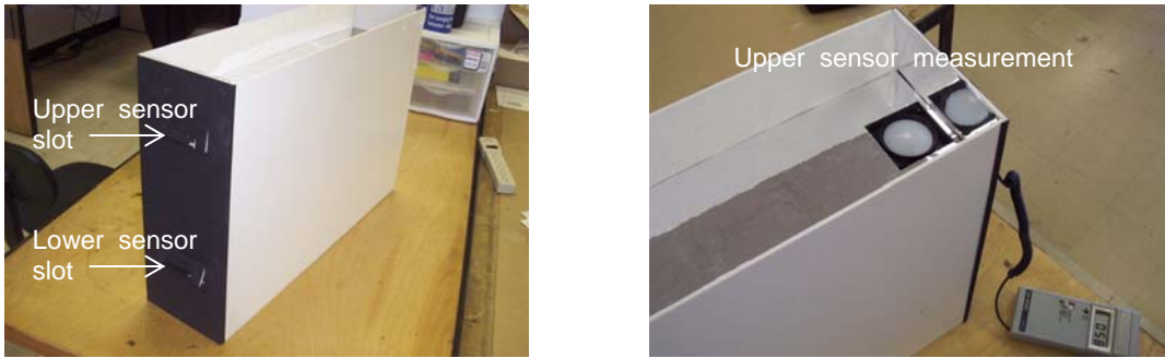
Figure 3.11: The sensor positions and diffuser area in the scale model test
