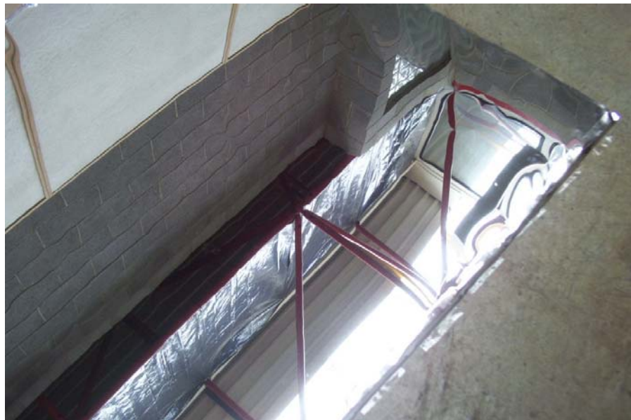
Figure 3.25: Tightening the specular film on the top cardboard layer by taping at both opposite sites along the length of the piece of enclosure
