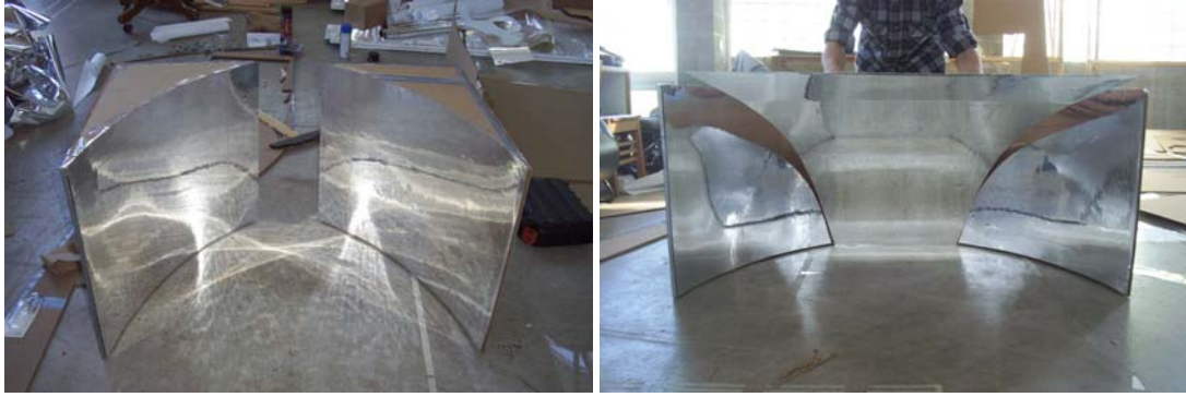
Figure 3.31: The demonstration of the reflection effect on the camera's flash (Left), and the completed assembling of the 3-piece back reflector (Right).
