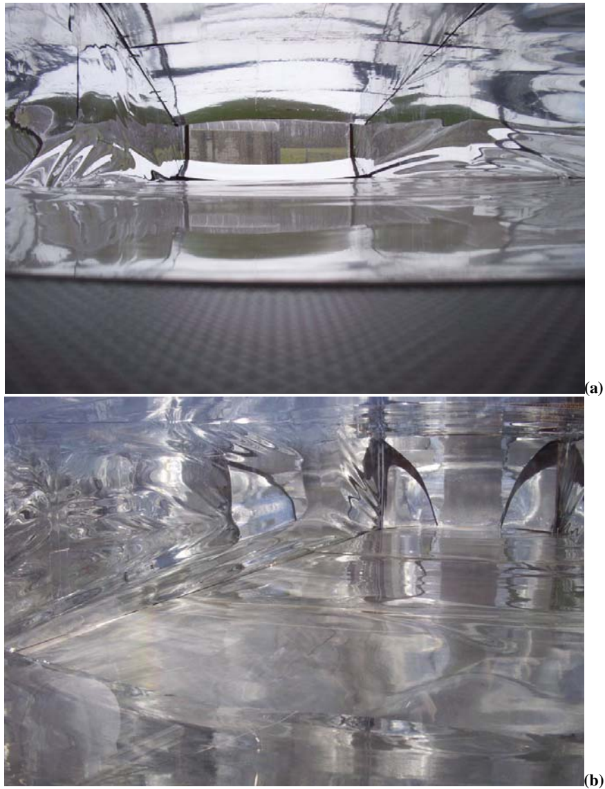
Figure 3.32: The images inside the cavity after installing the Multi-Curvature Geometric System ; (a) is the view looking from the diffuser to the inlet aperture, and vice versa (b)
