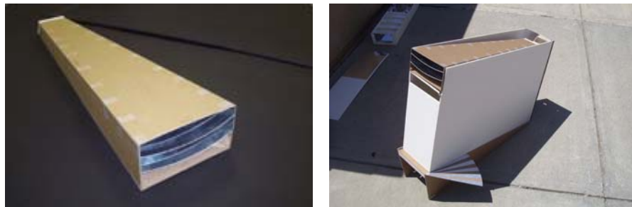
Figure 3.8: Tapered Geometric System with seasonal louvers
