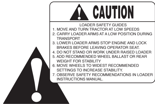
Figure 1. Typical safety sign for front-end loaders.
