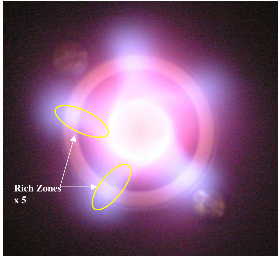
Figure 3.20. Picture of flame looking down the premixer. The five rich zones that were predicted by the CFD are easily distinguishable. Photo by author, 2010.
