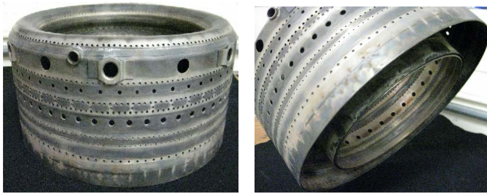
Figure 4.1. Original combustor liner for the PT6 turboprop engine using Jet-A fuel. Photos by Dan Villarreal, 2009, used with permission.
