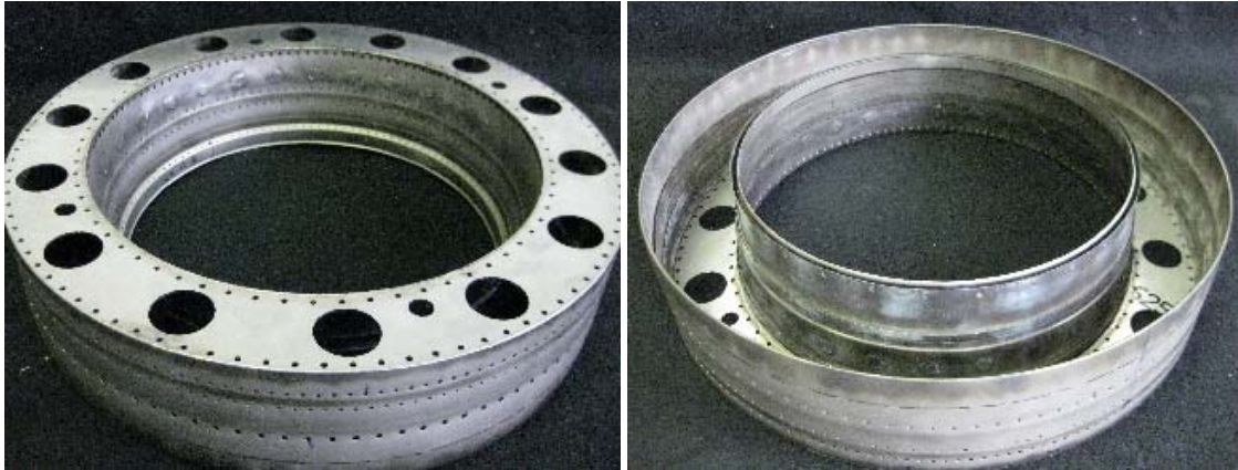
Figure 4.10. Lean premixed hydrogen combustor liner. Photos by author, 2009.
