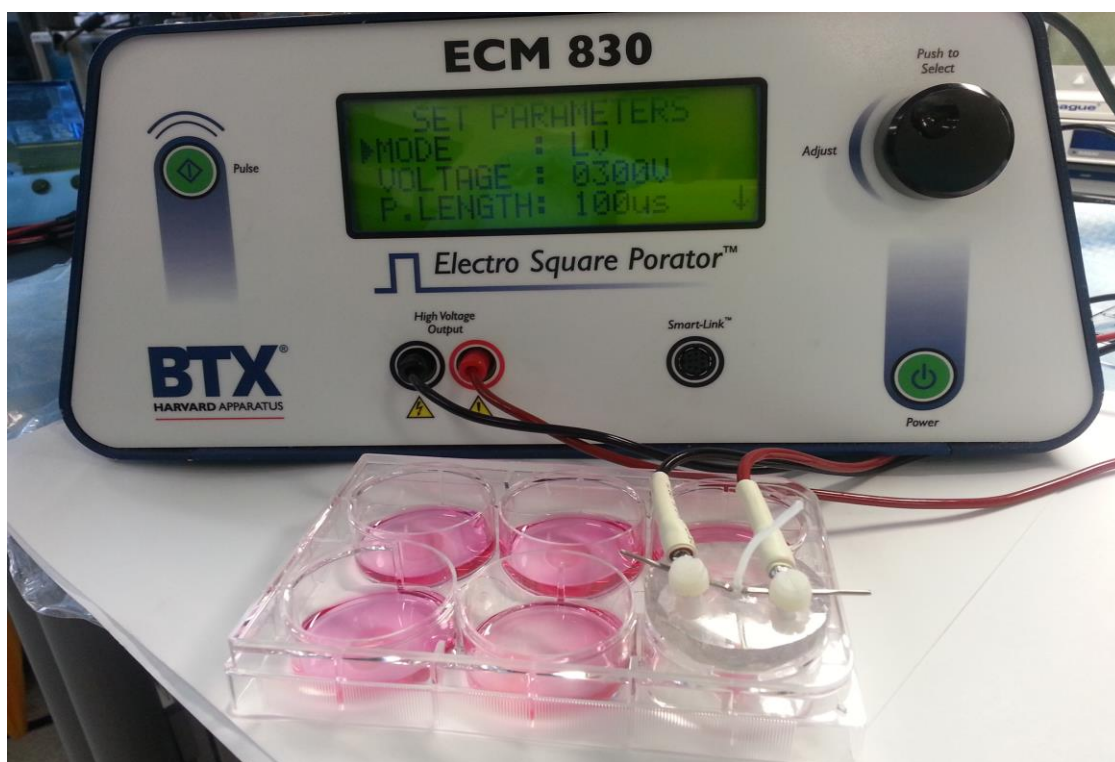
Figure 10: Hydrogel experimental setup with 6 well plate, electrodes, and BTX.
