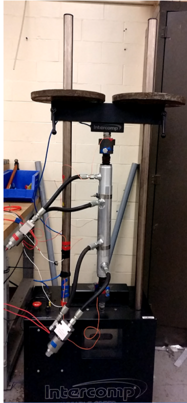
Figure 4.15: Application of Normal Load on the Shock Dyno.
