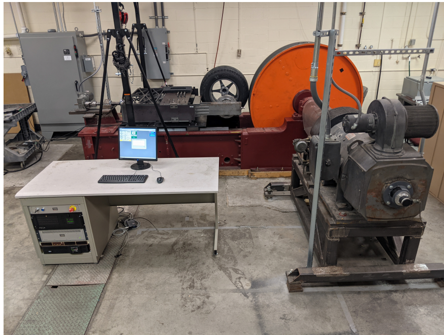
Figure 10.2: Rolling Resistance Machine Setup
