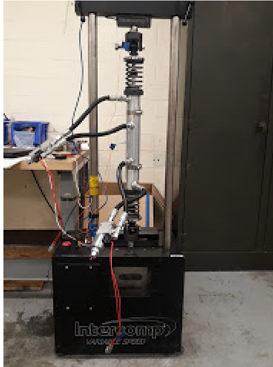
Figure 4.11: Double Damper with springs system mounted on the Shock Dyno.
