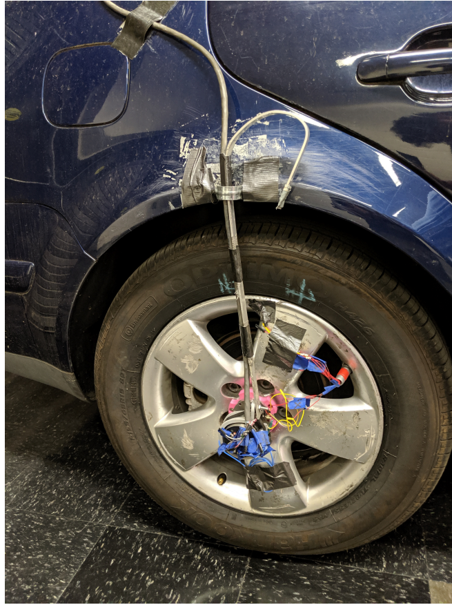
Figure 5.6: Slip Ring Assembly mounted on the wheel
