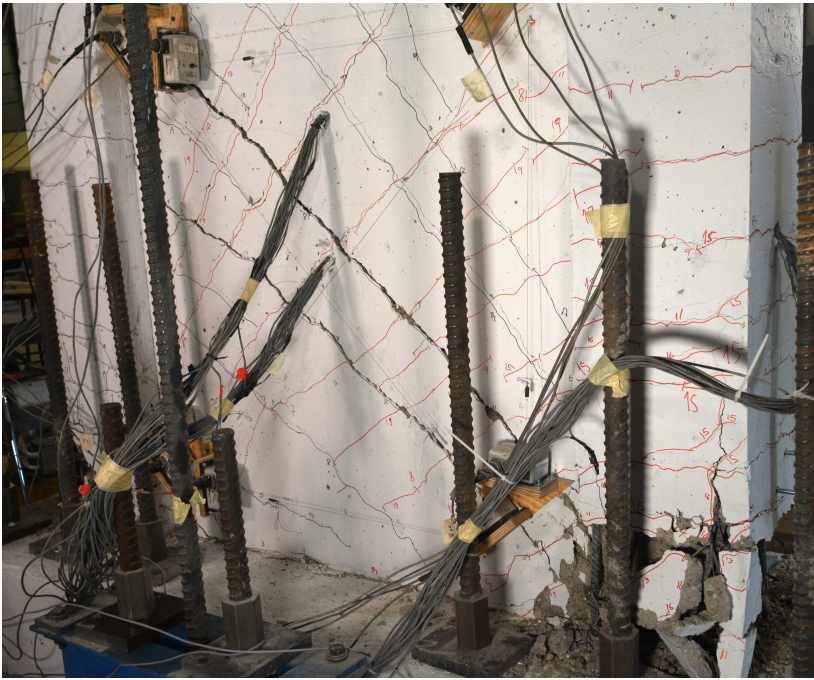
Figure 4.19: Back Lower Wall Final State of Specimen S1FW
