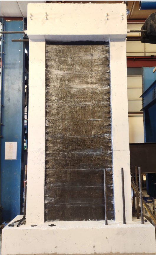
Figure 3.13: Specimen S1FW: Finished FRP Installation
