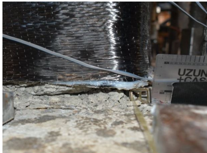
Figure 4.48: Final Toe Concrete Condition of Specimen S2FL
