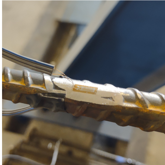
Figure 3.23: Strain Gauge on Reinforcement
