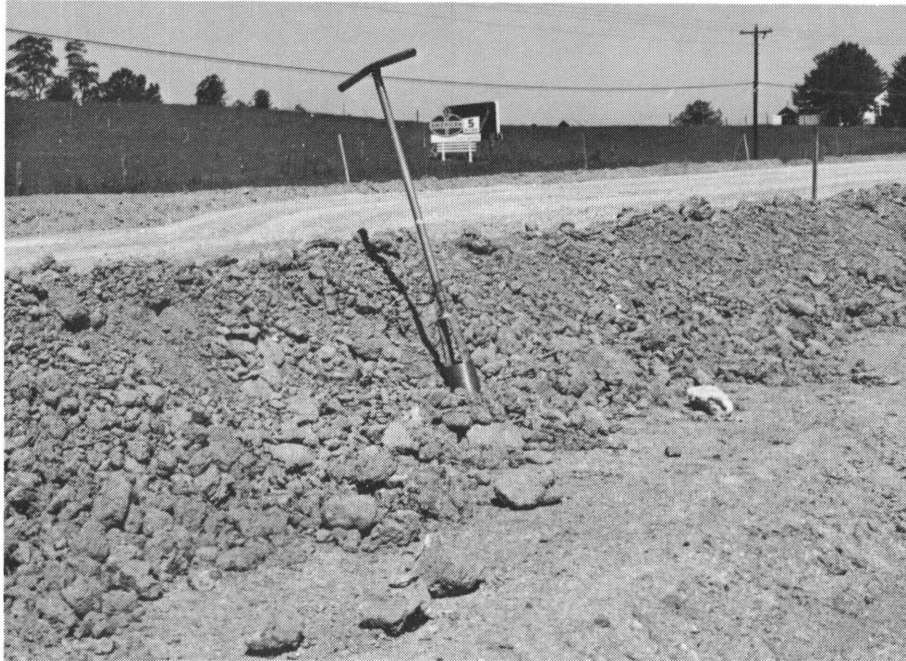
Plate 11. Clods from the subsoil of Lodi loam. The subsoil contains clays with shrink-swell properties which make compaction for road material difficult.
