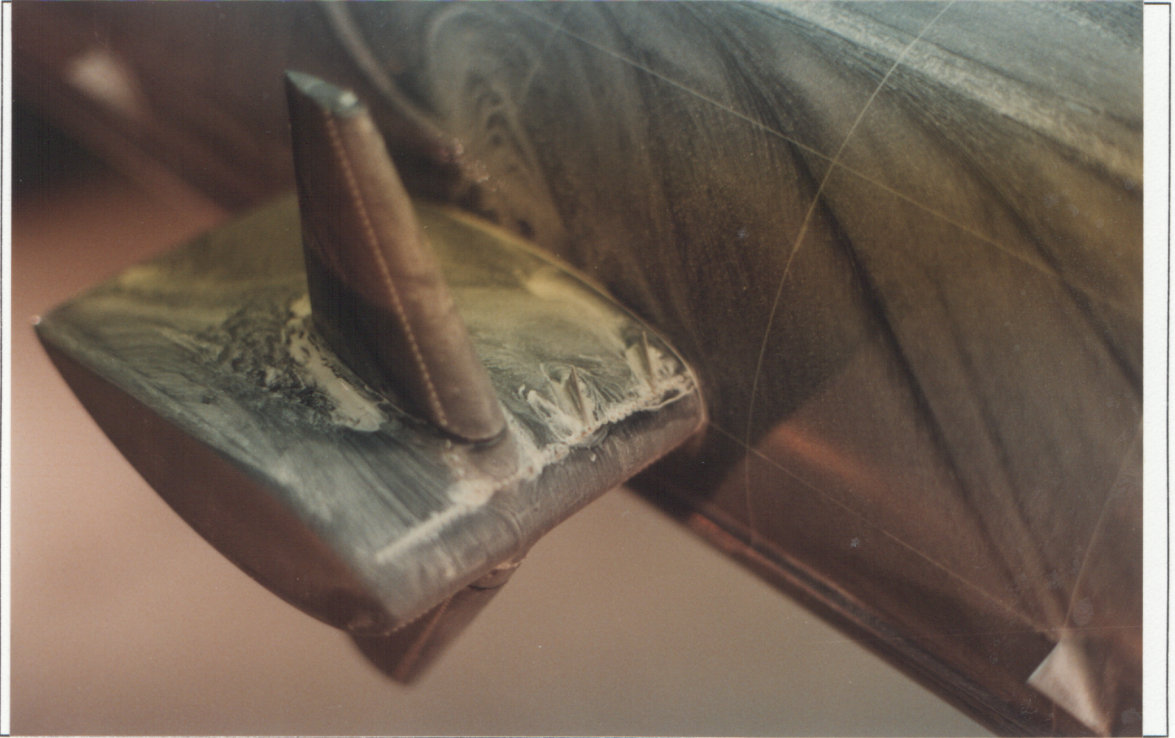
Figure 46. Fins on sail. Oil flow 23, Model 1, submarine with fins, \beta=15^\circ , Re = 6.7 million.
