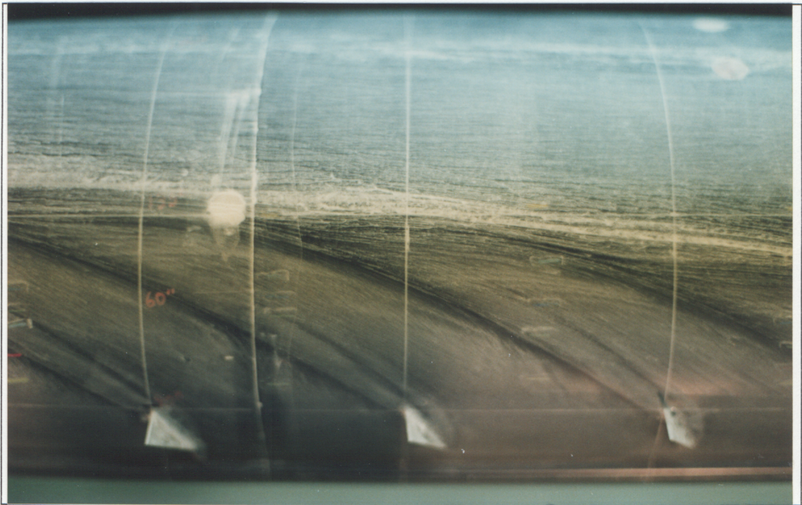
Figure 53. Oil flow 18, Model 1, submarine with fins, \beta=15^\circ , Re = 6.4 million.
