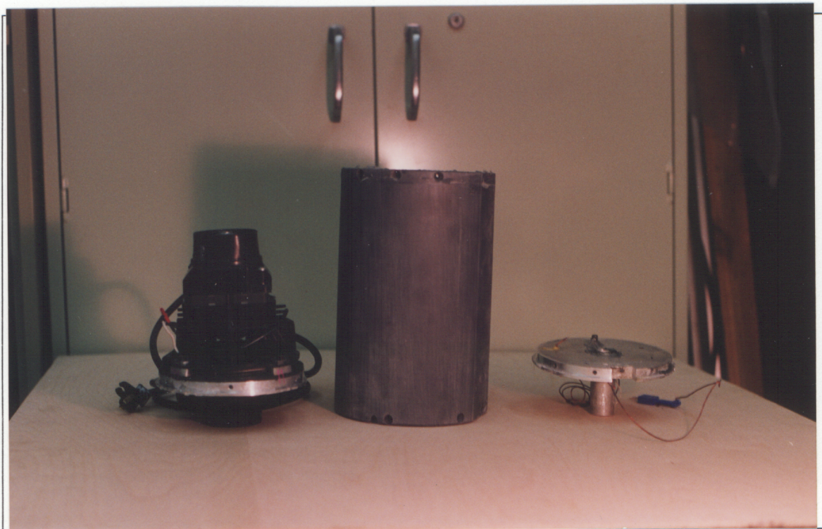
Figure 17. Fan motor (left), housing (middle), and end plate(right). End plate has pressure transducer and thermocouple embedded in it.
