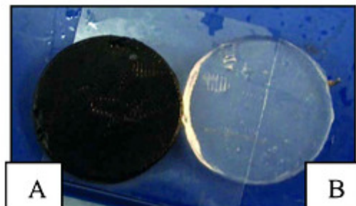
Figure 6.2: Sodium alginate phantom (a) with MWNT inclusion and (b) without MWNTs
