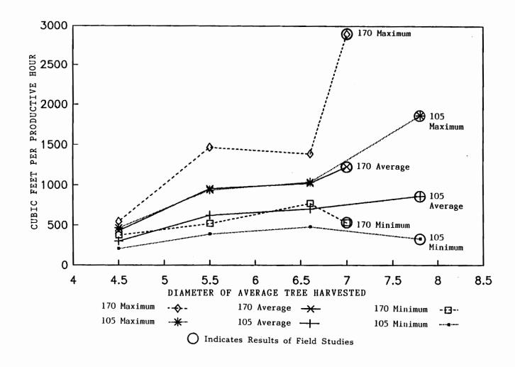
Figure 8. Productivity versus diameter of average tree harvested
