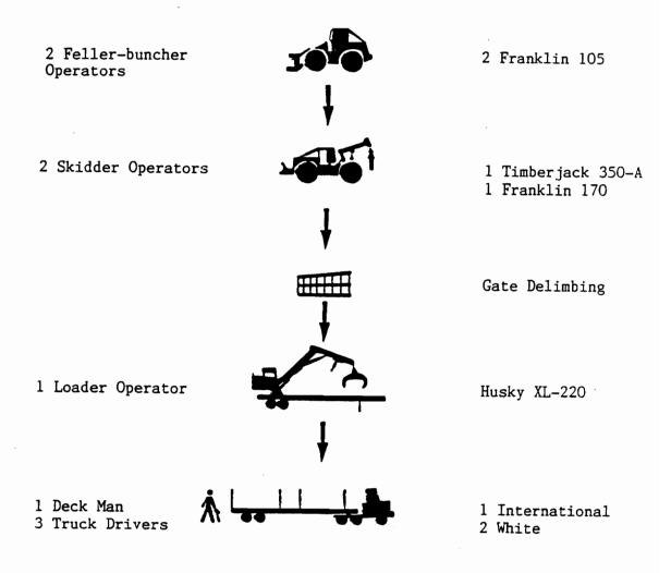
Figure 3. System B material flow.
