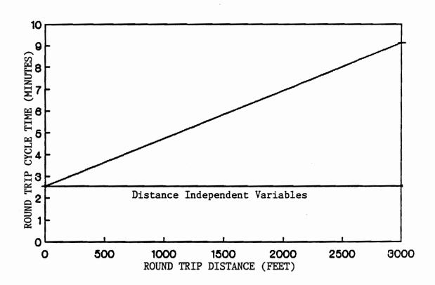
Figure 6. Graphic representation of round trip cycle time for Franklin 170 grapple skidder.
