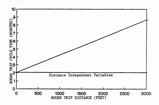
Figure 5. Graphic representation of round trip cycle time for Franklin 105 grapple skidder.
