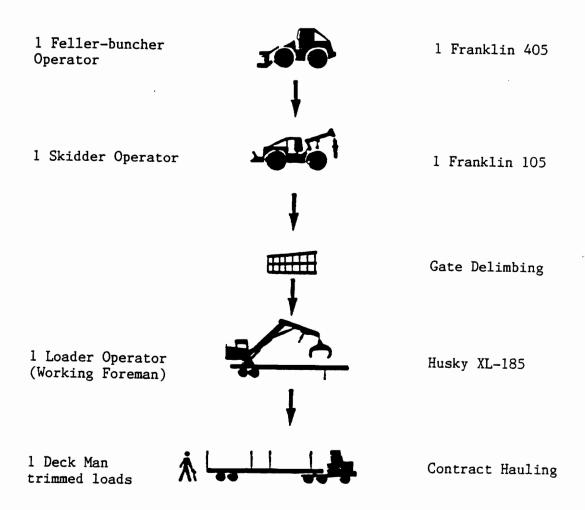
Figure 1. System A material flow.
