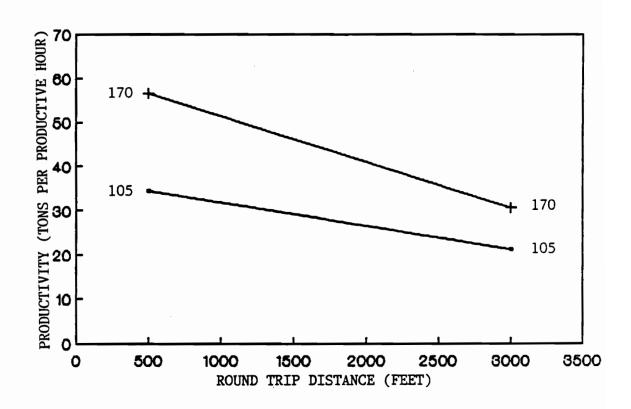
Figure 7. Graphical representation of productivity for the 105 and 170.
