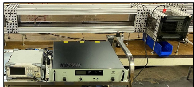
Fig. 3 Vibratory instrument: waveform generator (left), power amplifier (middle), electro-mechanic shaker (right)
