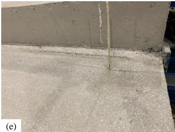
Figure 3.15. Photos of Construction Progression: (a) Shoring Erection; (b) Reaction Truss in Position; (c) Specimens Ready to Cast; (d) Specimens Cured; (e) Surface Grinded; (f) Externally Bonded FRP System Installed.
