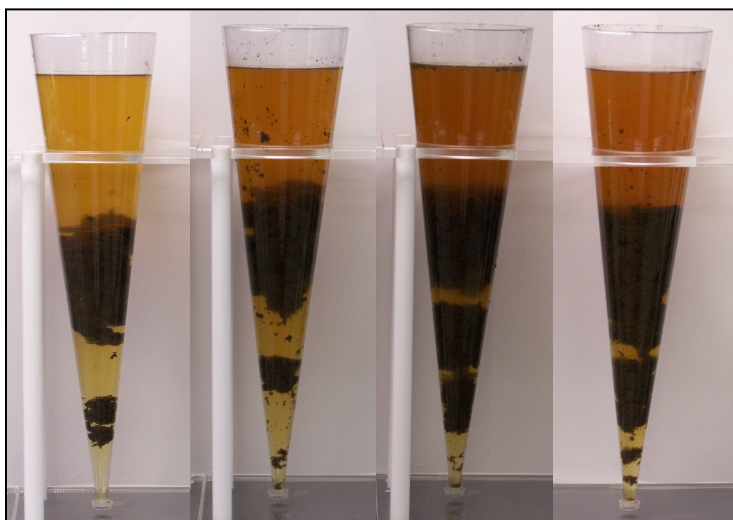
Figure 15. Using treated supernatant as dilution water resulted in successively darker supernatants and less sludge compaction. Dilution 1 (as previously defined) is shown at left, followed by Dilution 2, Dilution 3, and Dilution 4 (far right). The samples shown received alum dosages of 180 mg Al/L and 4512 dosages of 100 mg/L.
