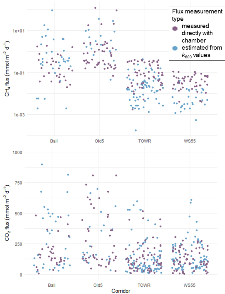
Figure S1. Comparison of measured and estimated flux values. Measured values come from chamber placements. Estimated values come from k_{600} values derived from the chambers that were then applied to dissolved gas concentrations (equation 3 in main text).
