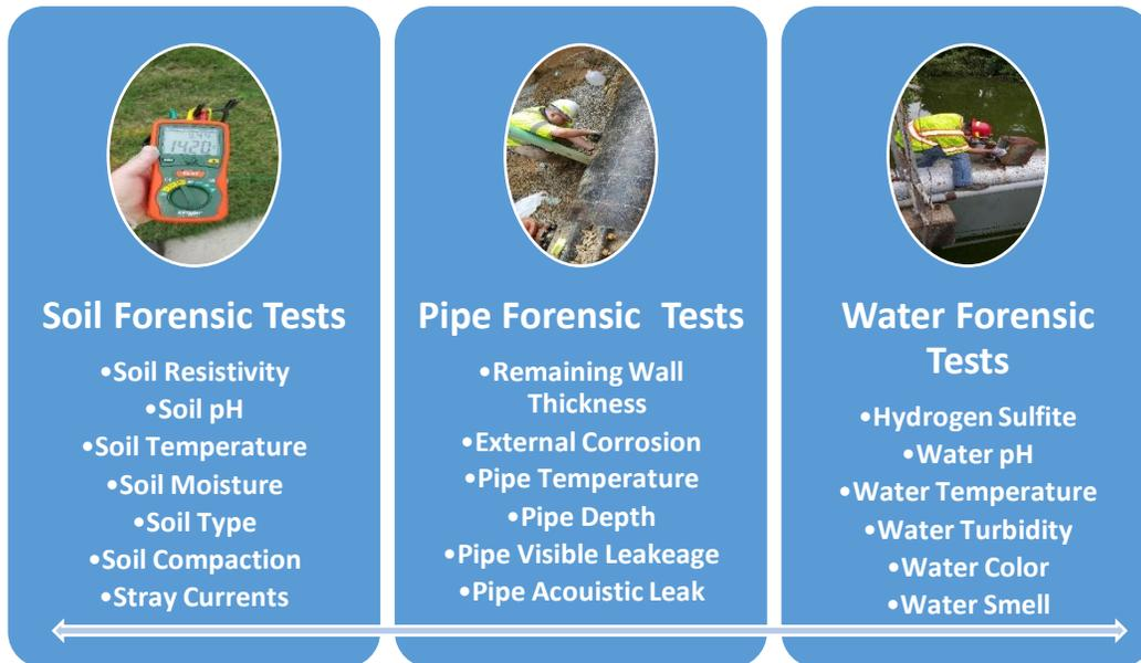
**Figure 5-17. Forensic Tests for the Piloting Sites**
