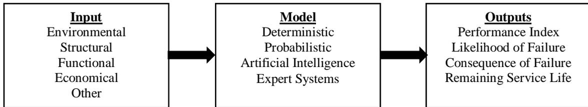
**Figure 2-5. Wastewater Pipeline Performance Prediction Models**
