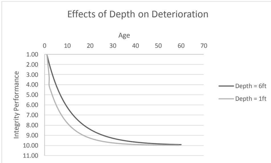
**Figure 6-8. Example State Dependent Deterioration Curve with Ordered Logistic Regression.**
