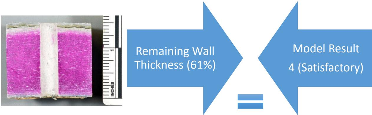
**Figure 5-20. Piloting Site #3, Ground Truth and Index Results Agree.**
