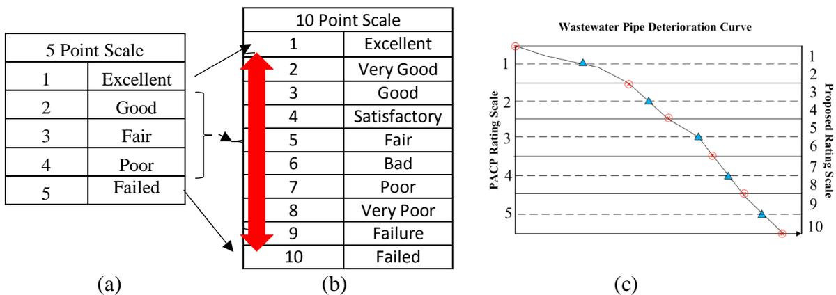
**Figure 5-5. 5-Point Scale vs. Proposed 10-Point Scale for Performance Prediction**
