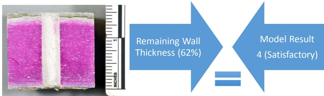
**Figure 5-18. Piloting Site #1, Ground Truth and Index Results Agree.**
