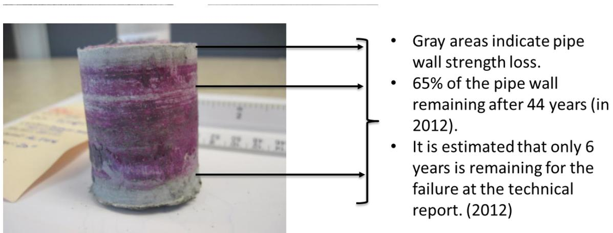
**Figure 5-14. Test Results for the Phenolphthalein Test.**
