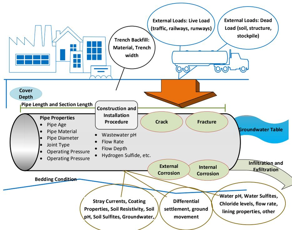
**Figure 1-1. Factors Effecting Wastewater Pipeline Performance**
