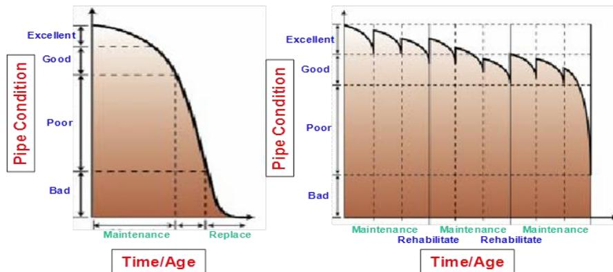
**Figure 2-3. Condition/Performance Deterioration Prediction Model.**
