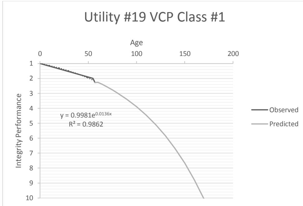
**Figure G19-5. Time Dependent Model for Utility #19 VC pipe class #1 (collection, less than 24” diameter, construction era 1955 to 1975).**
