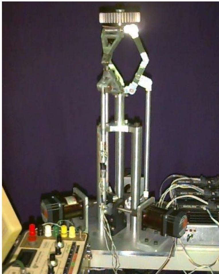
Figure 5.5: Dynamic Force Measurement System
