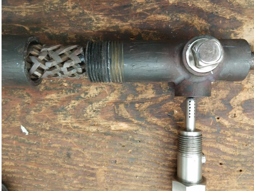
Figure 2.1: The phase distributor used for the work presented in this dissertation.
