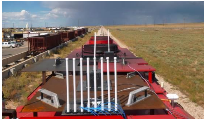
Figure 3 Antenna installations for TTCI
