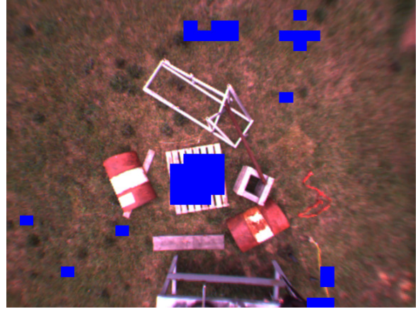
Figure 27: A simulated descent, at a height of 2.44 meters with acceptable landing sites overlaid.
