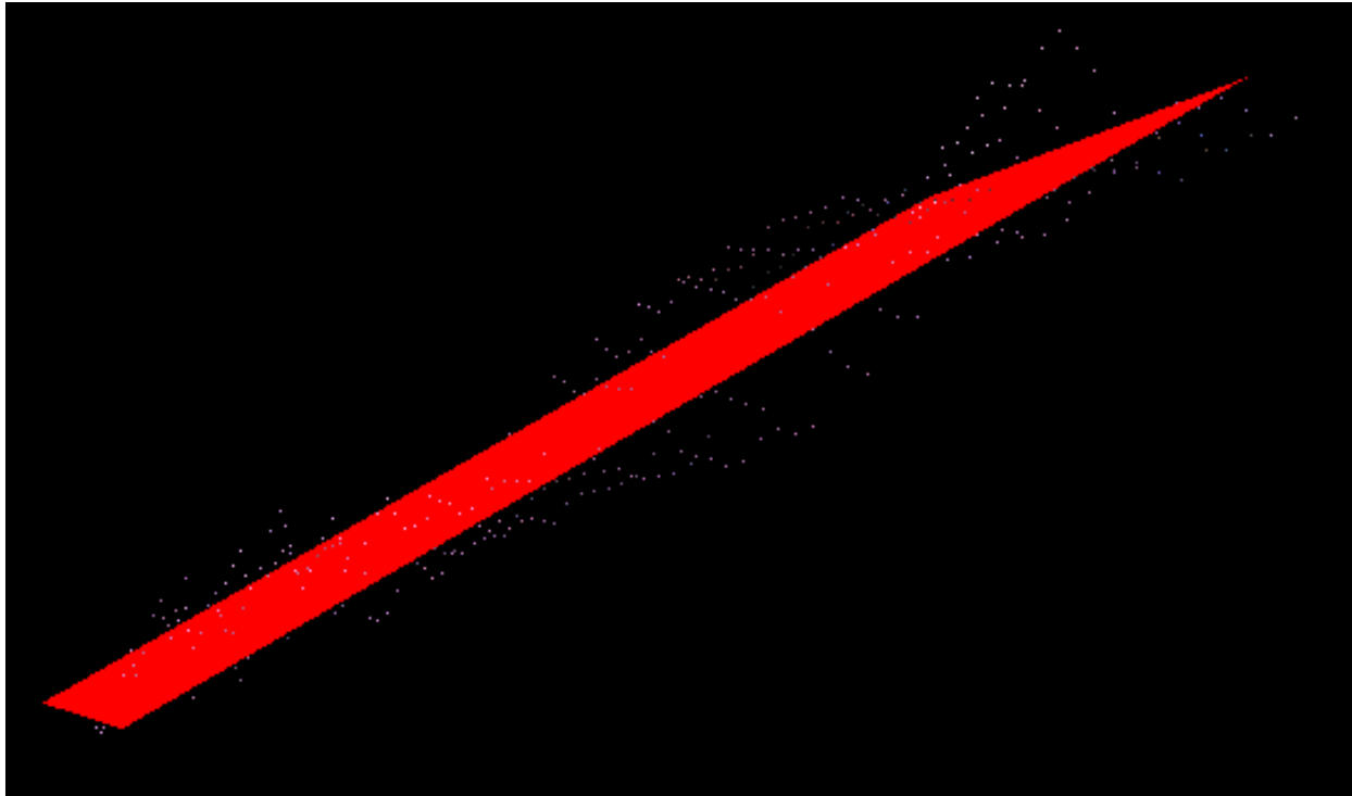
Figure 17: A sample best-fit plane and its corresponding data points.
