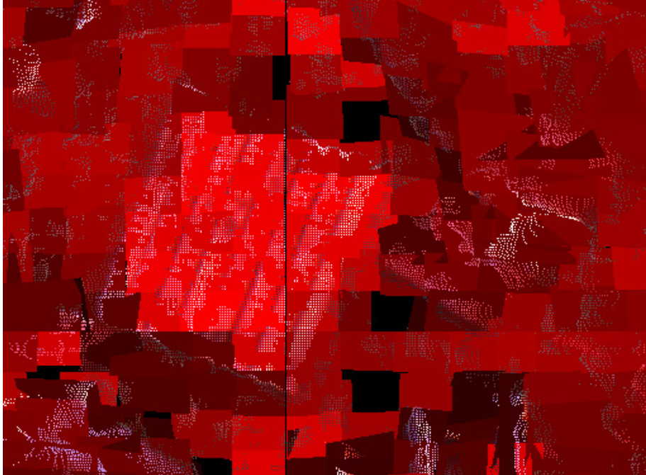
Figure 39: A point cloud with best-fit planes overlaid. The planes are colored according to their slope (in comparison to the vertical direction). Flat planes appear lighter, while steep planes appear darker.
