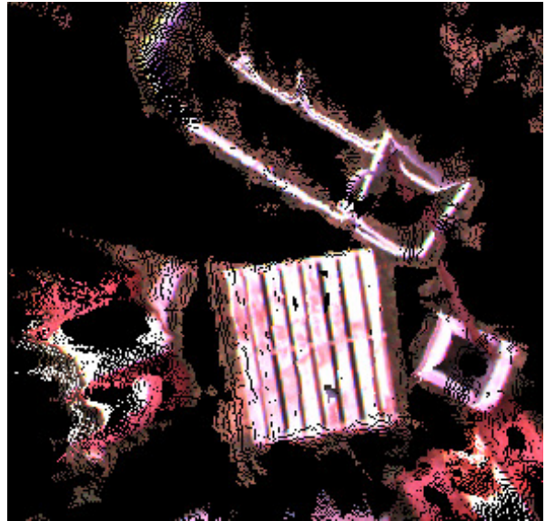
Figure 23: The point cloud of the example scene, obtained using images from the Bumblebee stereo vision camera system.
