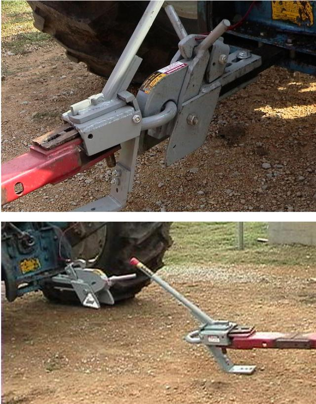
Figure 11. Quick-connect adaptor for attaching implements to drawbar. Farmer remains in the operator's seat and does not dismount for hitching and unhitching the implement.
