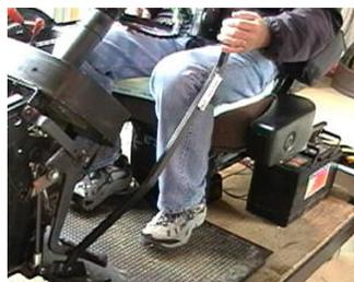
Figure 8. Modified tractor controls for operators with disabilities: (upper left) tractor controls on the right to accommodate a left-hand amputee; (upper right) spinner knob for steering wheels for better grip and one-hand steering; (lower) hand levers for brake engagement for limited leg mobility or strength.
