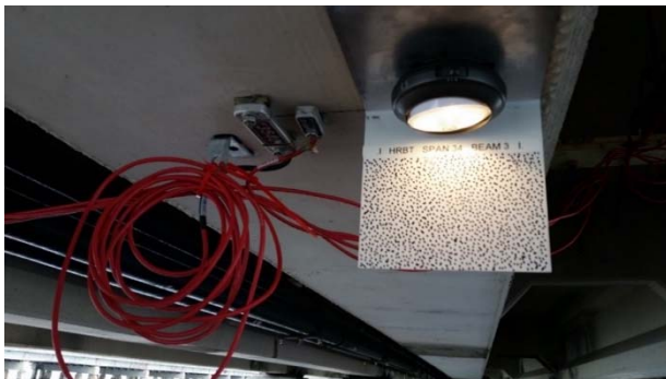
a) DIC Target Card with Local Lighting
