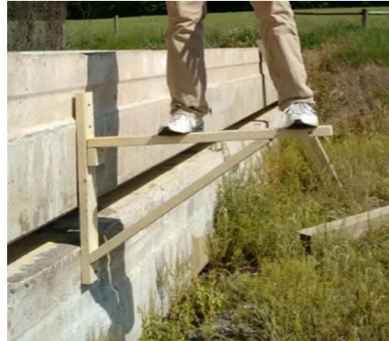
b) Proof Testing Single Outrigger
