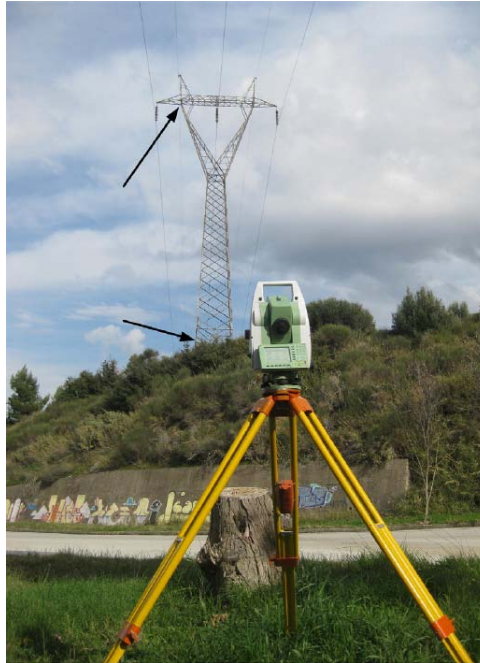
Figure 12: Robotic Total Station System (Moschas and Stiros 2014)
