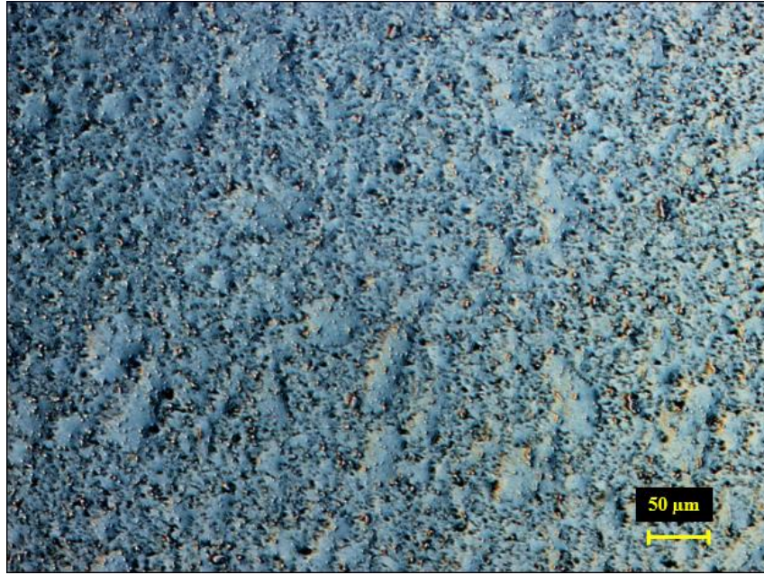
Figure 6.17: Optical micrograph of a composite of Co with 10 vol.% \text{Co}_{60}\text{C}_{40} after being attritor milled for 2 hour then SPSed by 300 MPa for 10 minutes at 350°C. Grey areas are composite of Co matrix and \text{Co}_{60}\text{C}_{40} particles while black areas are pores. Photomicrograph is shown at 20X.
