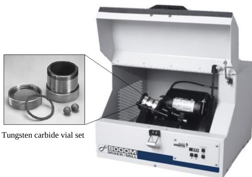
Figure 3.3: SPEX 8000M Mixer/Mill® with a tungsten carbide vial set.
