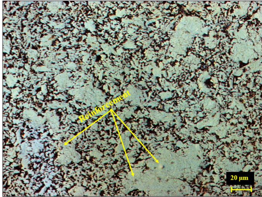
Figure 6.7: Optical micrograph of a composite of Co with 1 vol.% \text{Co}_{60}\text{C}_{40} after being attritor milled for 2 hour then SPSed by 300 MPa for 10 minutes at 350°C. Grey areas are composite of Co matrix and \text{Co}_{60}\text{C}_{40} particles while black areas are pores. Photomicrograph is shown at 50X.
