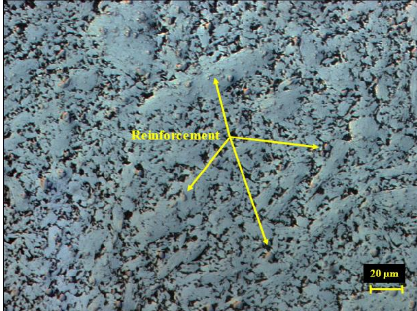
Figure 6.24: Optical micrograph of a composite of Co with 20 vol.% \text{Co}_{60}\text{C}_{40} after being attritor milled for 2 hour then SPSed by 300 MPa for 10 minutes at 350°C. Grey areas are composite of Co matrix and \text{Co}_{60}\text{C}_{40} particles while black areas are pores. Photomicrograph is shown at 50X.
