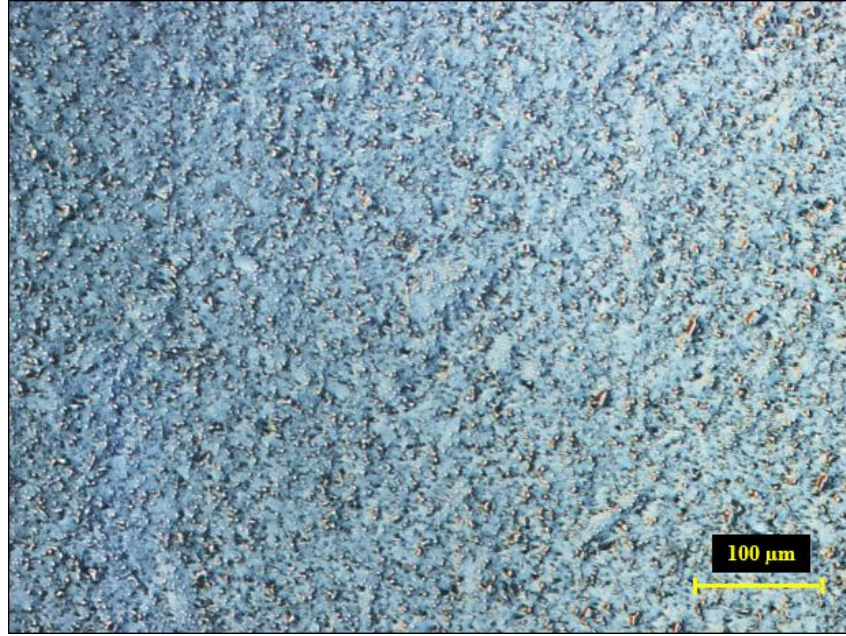
Figure 6.23: Optical micrograph of a composite of Co with 20 vol.% \text{Co}_{60}\text{C}_{40} after being attritor milled for 2 hour then SPSed by 300 MPa for 10 minutes at 350°C. Grey areas are composite of Co matrix and \text{Co}_{60}\text{C}_{40} particles while black areas are pores. Photomicrograph is shown at 20X.
