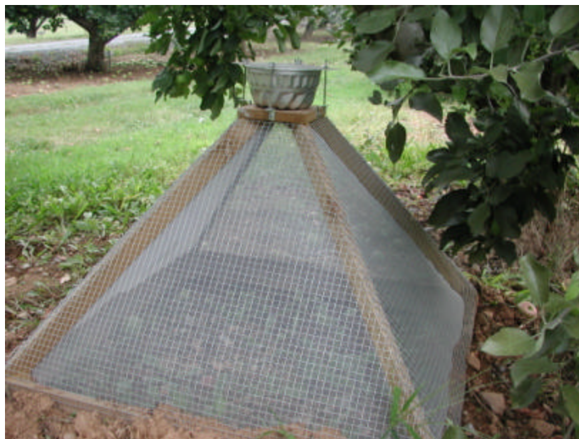
Fig. 8. Emergence trap used in 2002.
