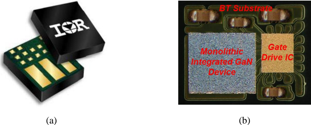
Fig. 2.33: (a) IR GaN-based integrated power stage devices (b) device interior
