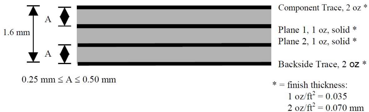
Fig. 4.6: Cross section of multi-layer PCB showing trace and dielectric thicknesses
