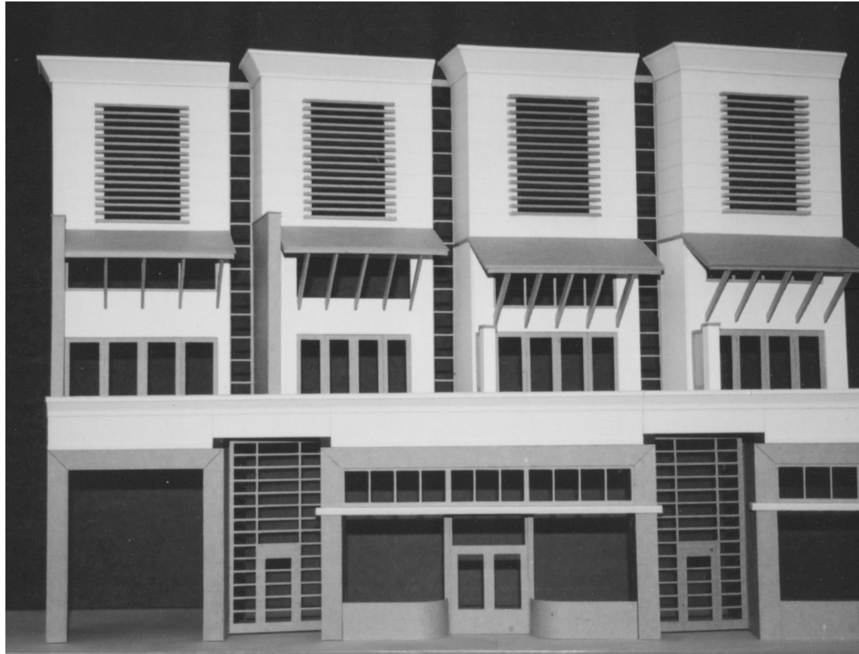
above: Photograph of model showing misalignment of vertical elements.
