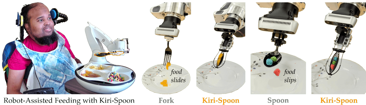
Figure 1.2: Kiri-Spoon is a spoon-shaped kirigami utensil specifically designed for robot-assisted feeding. (Left) Robot arms equipped with Kiri-Spoon can robustly acquire foods from the plate, safely carry those morsels to the human, and then seamlessly transfer items into the user’s mouth. (Right) It is challenging for robot arms to dexterously manipulate traditional utensils such as forks and spoons. By comparison, Kiri-Spoon makes the robot’s task fundamentally easier by flexibly wrapping around the desired foods. This capability enables Kiri-Spoon to function as a fork (pinching foods) or as a spoon (scooping foods).
