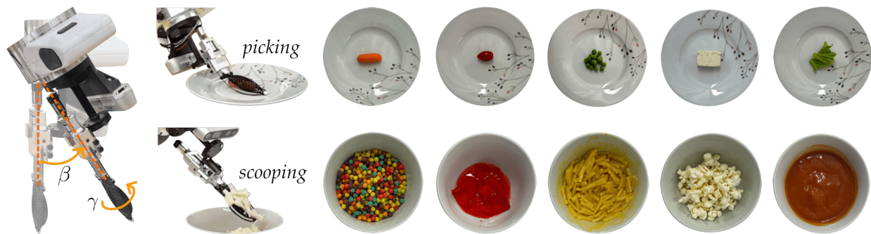
Figure 4.6: Experimental setup for the autonomous tests in Section 4.3. (Left) Position and orientation of Kiri-Spoon during autonomous acquisition. When picking foods from a plate, the flexible hoop and kirigami sheet bend to align with the orientation of that plate. Upon reaching the target position, we rapidly increase the curvature of the kirigami sheet to firmly grasp the desired food. In contrast, Kiri-Spoon maintains a spoon-like curvature when scooping food from a bowl. (Right) Foods used in our acquisition experiments. For picking, we include round foods of different sizes, i.e., carrots, cherry tomatoes, and peas. We also test with soft and slippery foods like silken tofu and flat foods like lettuce. For scooping, we include dry foods like cereal and popcorn, sticky foods like macaroni and cheese, slippery foods like jello, and liquid foods like tomato soup.
