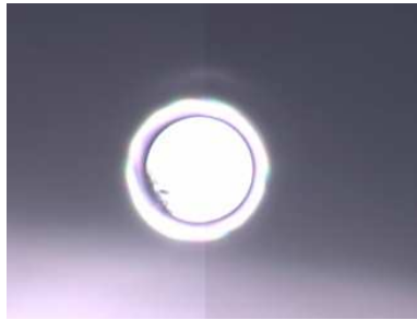
Figure 6.4: Sensor's endface view photo taken from a microscope (Zeiss Axiovert 25).
