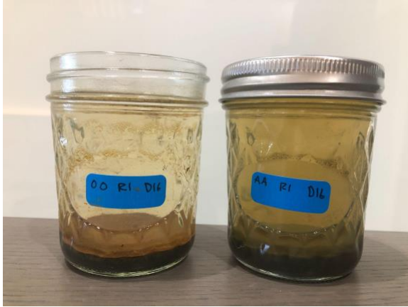
Figure S2. Photo illustrating experimental microcosm set-up, with visual differences between treatments on day 13 of the experiment. Left: an oxic microcosm. Right: a hypoxic (sealed) microcosm. Note that the oxic microcosm has an orange biofilm overlying sediment, suggestive of oxidized Fe, while sediments and water in the hypoxic microcosm are darker, suggestive of reduced Fe. Microcosm containers were 177 mL glass jars with two-piece gasket-sealed lids (Verones brand).
