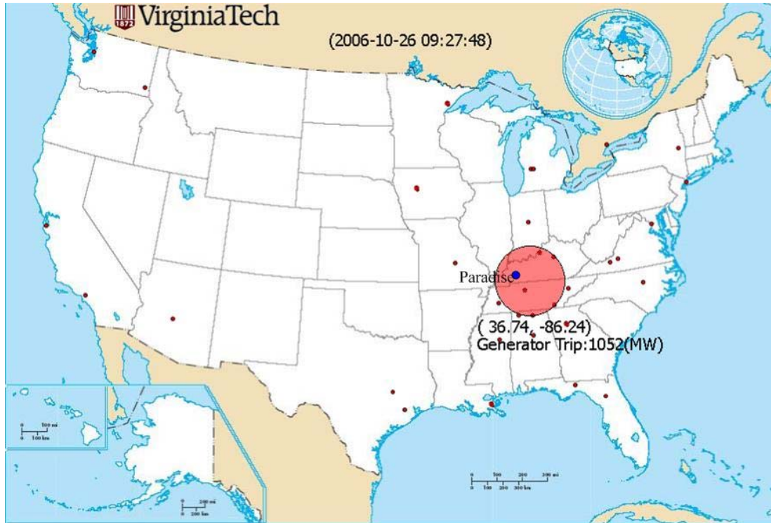
Figure 6.19 The estimated disturbance location of the example. (The estimated location is shown as the red circle. The real location is shown as the blue dot. Map source: USGS)
