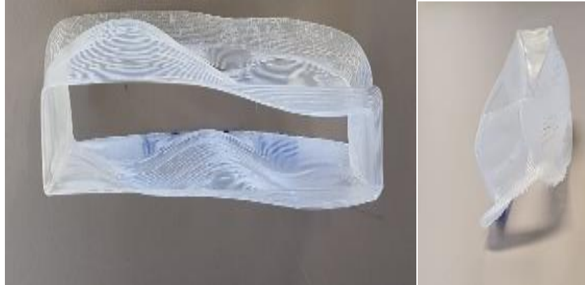
Figure 12. Structural deformation and warpage in a thin-walled PP2 structure. Left: top view, right: side view
