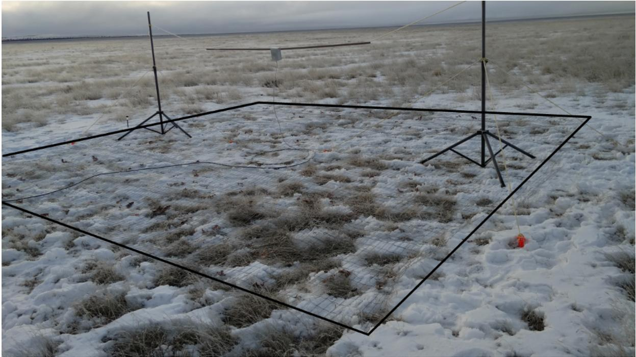
Figure 3.2: Deployed antenna, with the ground screen outlined. See Fig. 3.4 for dimensions.
