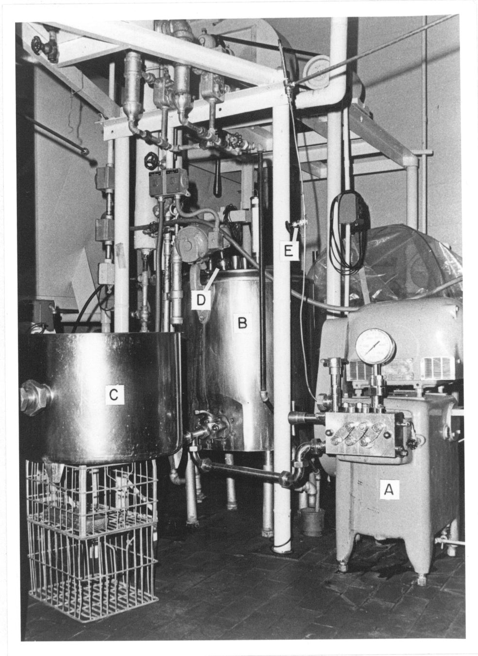
Fig. 4 - High pressure pump and mixing vats for high-solids products. A, high pressure pump; B, product vat; C, water vat; D, mechanical stirrer; E, sampling valve No. 1.
