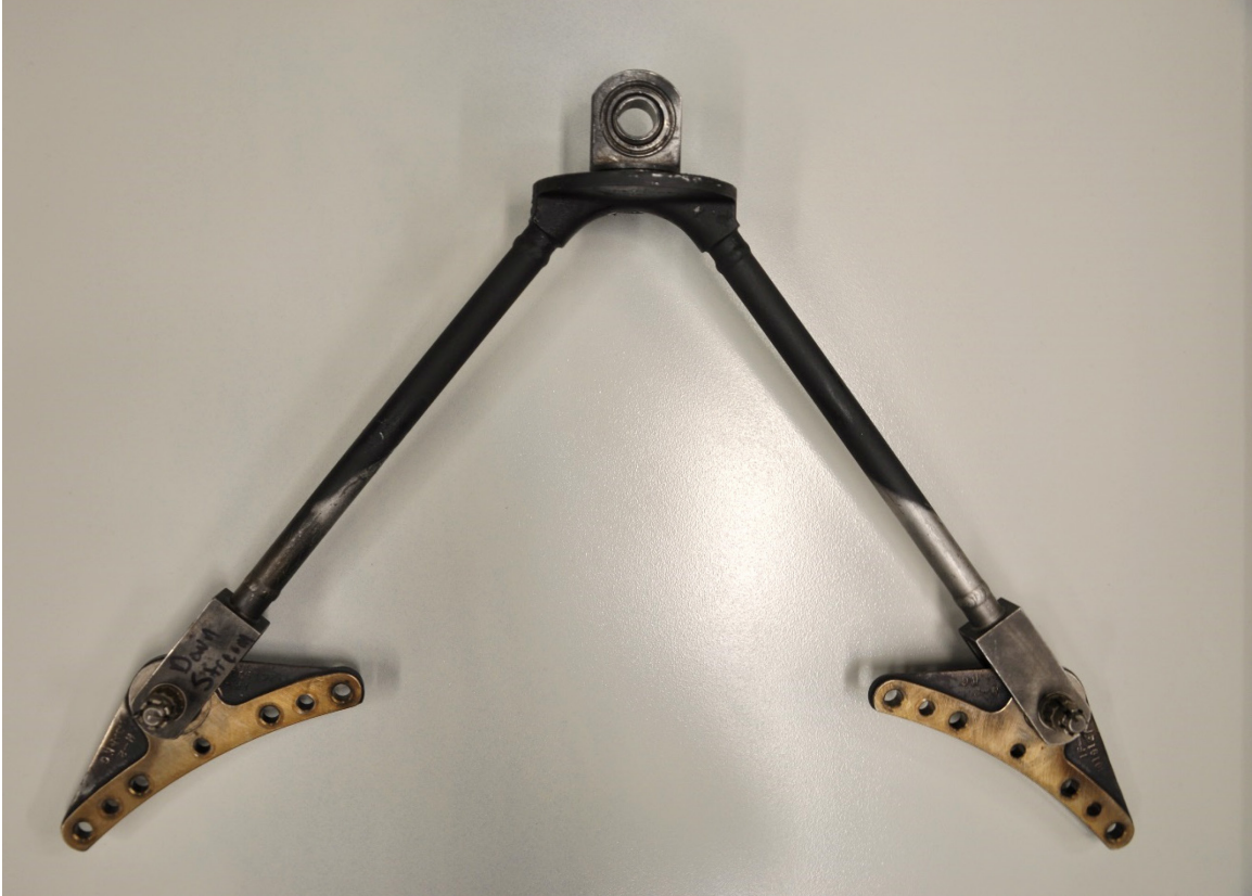
Figure 19 – Aft support strut removed from the JT15D-1 engine
