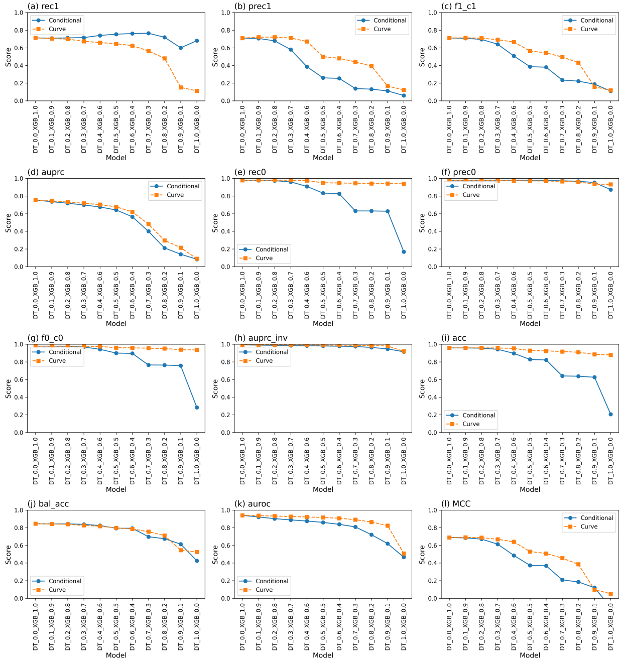
Figure 4.19: Performance of XGBoost and Knowledge-based Decision Tree combined model. Each subfigure demonstrates the performance of different combinations of merge coefficients starting from 0 to 1 with step of 0.1. XGB_1.0 represents the original model performance, whereas DT_1.0 represents the Knowledge-based Decision Tree performance only.
