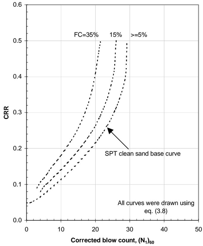
Figure 3.3 SPT clean-sand base curve for magnitude 7.5 earthquake
