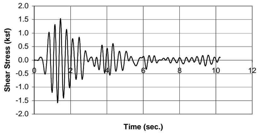
Figure 3.2 Example of shear stress time history during earthquake
