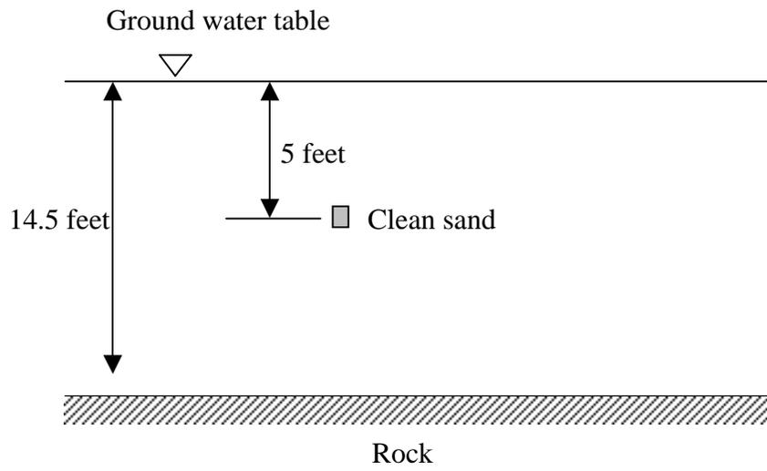
Figure 3.6 Soil profile for calculation example
