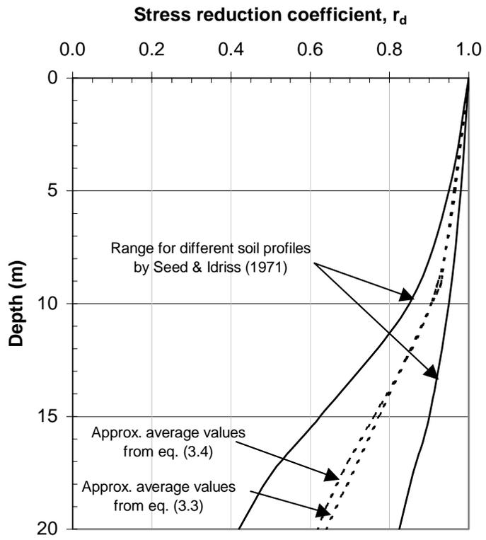
Figure 3.1 Values of stress reduction coefficient versus depth
