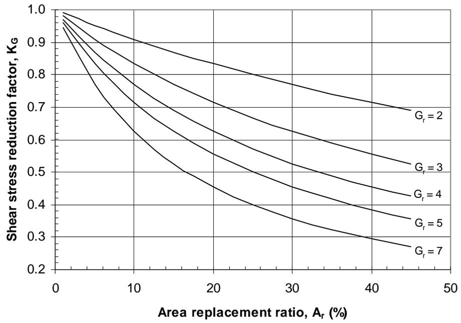
Figure 3.5 The shear stress reduction factor,  $K_G$  (after Baez and Martin, 1993, 1994)
