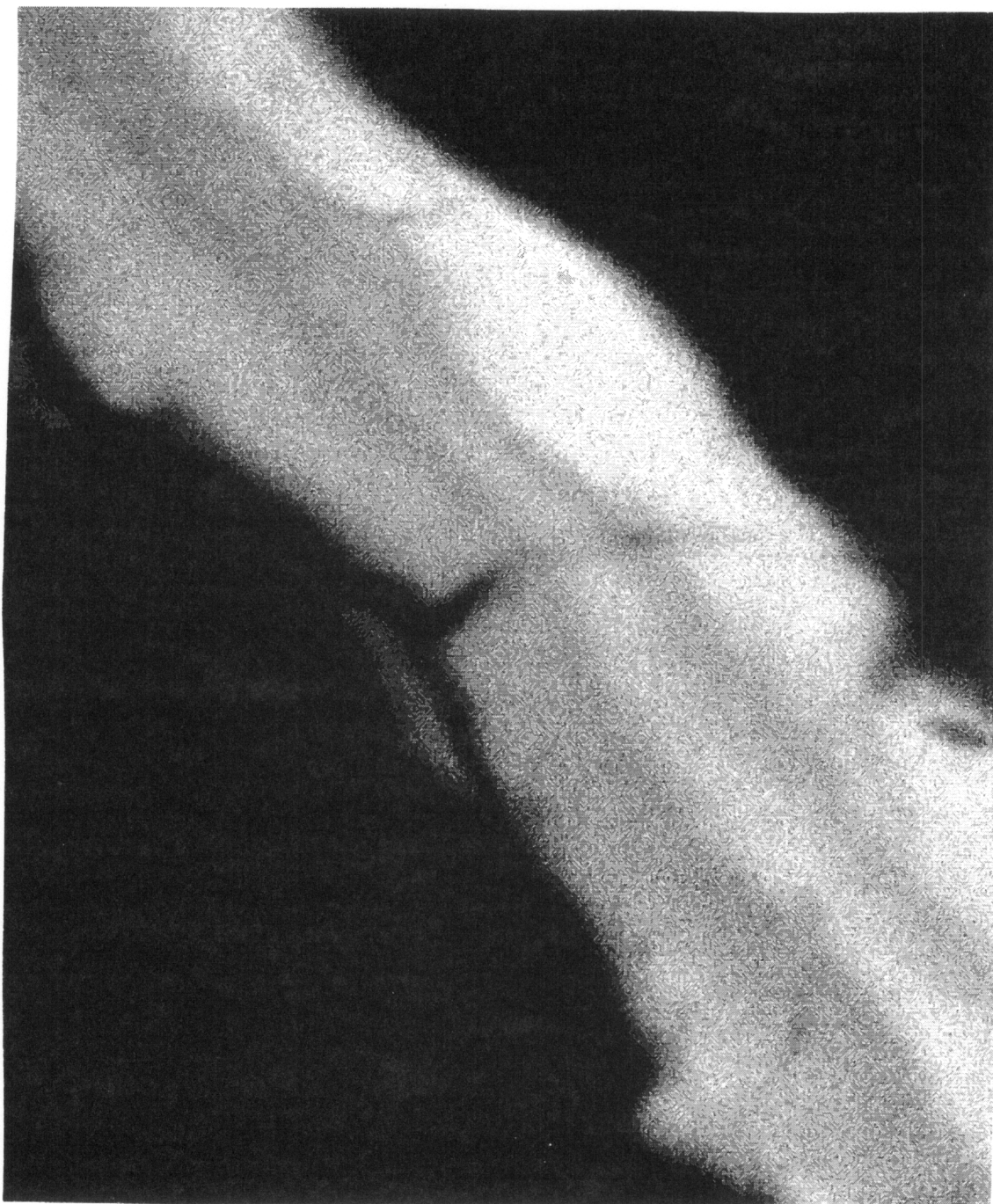
FIGURE 26 Areal map of Mn by electron microprobe analysis, Ft. Collins, CO facility oxide coating on anthracite (Nov. 1994 sample, polished cross section). Media grain is at left, coating outer surface at right. Vertical dimension of figure is 37.5 microns.
