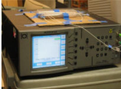
Figure 2-6 Photo of Component Testing System (CTS) used to monitor fabrication and static testing processes.
