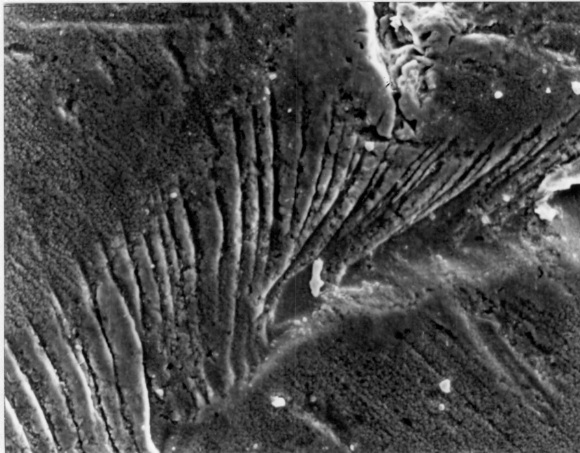
Figure 4.12 Slip bands observed on Cu-Ni specimen fatigued at 181 \mu\text{A}/\text{cm}^2 , anodic.
